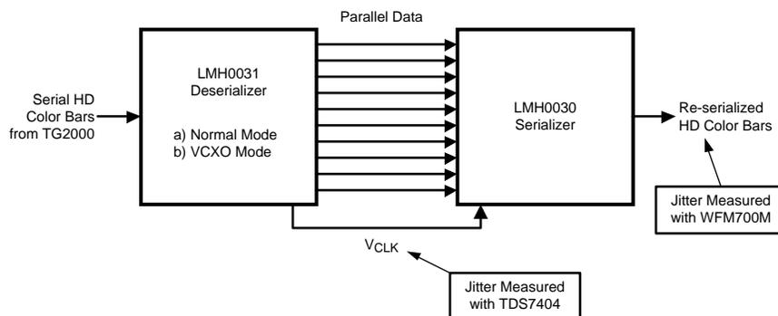
**Figure 2. Jitter Measurement Setup**
