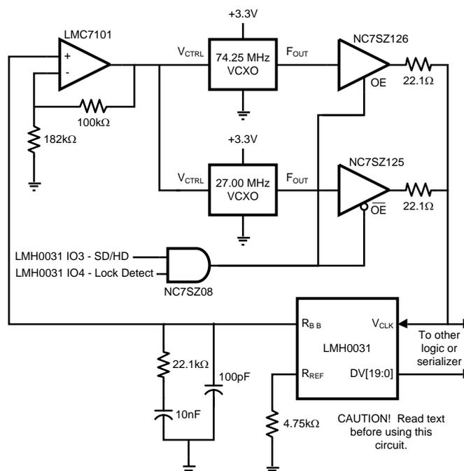
**Figure 1. Using Dual VCXOs for  $V_{CLK}$**
