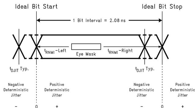
**Figure 3. Parameter Relationships to Generate the Eye Mask**
