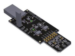
Figure 1. TMP392 Evaluation Board
