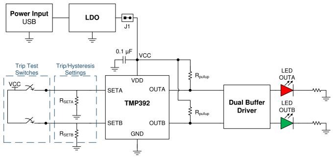
Figure 4. TMP392 Evaluation Board Block Diagram
