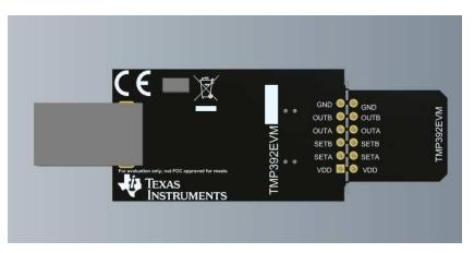
Figure 3. TMP392 Evaluation Board Bottom Side
