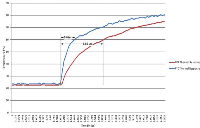
**Figure 3-3. Comparison of Response Speed Between TMP61 and NTC**
