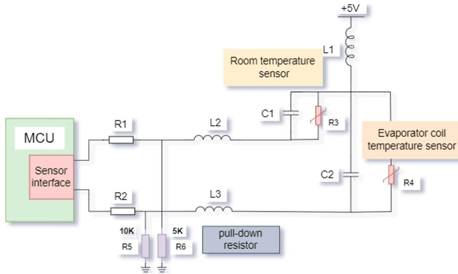
Figure 1-3. Schematic of the Temperature Sensor Circuit of the Indoor Unit
