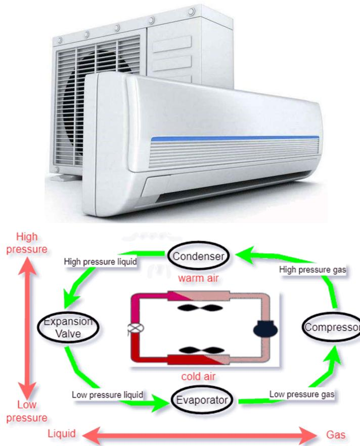
**Figure 1-1. Schematic Diagram of the Principle of Air Conditioning and Refrigeration**
