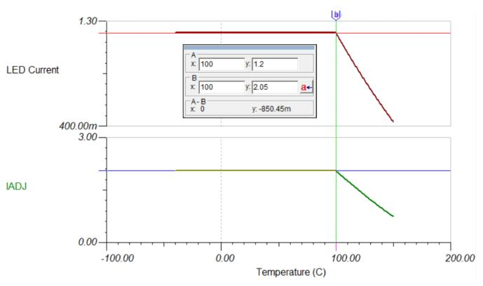
Figure 11. 100 °C Current Output Curve
