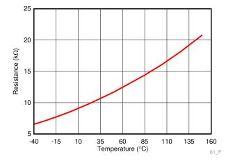
Figure 1. TMP61-Q1 Resistance Curve vs Temperature
