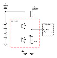
Figure 5. PTC-Conditioning Circuit
