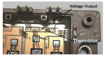
Figure 1. Thermistor in an IGBT Module
