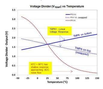
Figure 4. Voltage Biased Output of PTC vs NTC
