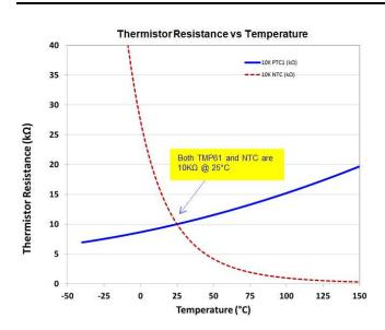
Figure 3. Resistance vs Temperature of PTC vs NTC
