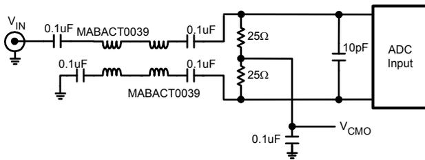
Figure 3. Analog Input Network for  $F_{IN} > 70\text{MHz}$
