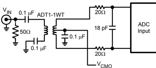
Figure 4. Analog Input Network for  $F_{IN} < 70\text{MHz}$
