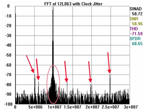
Figure 4a. Jitter causes spectral spreading and spurs
