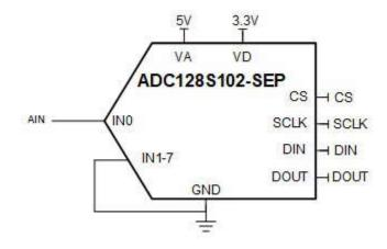
Figure 3-2. ADC128S102-SEP Bias Configuration
