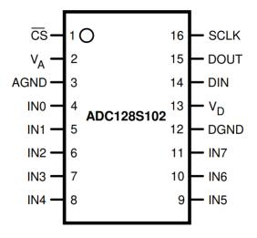
Figure 3-1. ADC128S102-SEP Pinout Diagram
