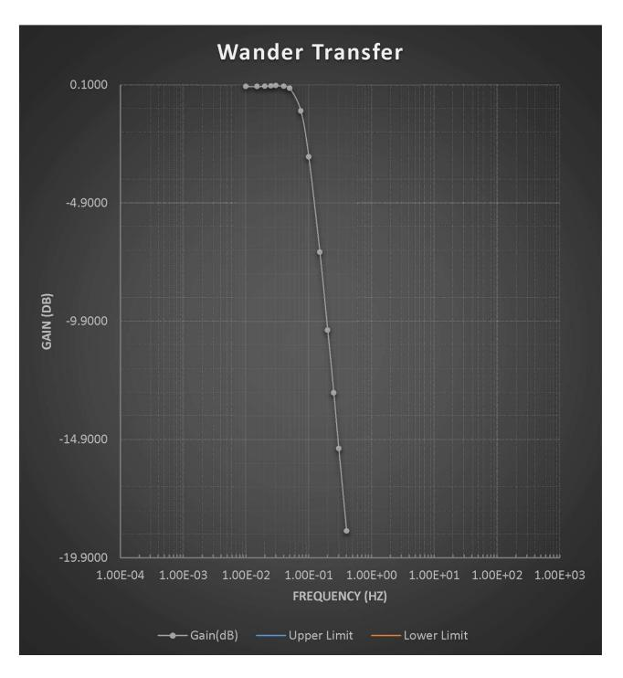
Figure 13. Wander Transfer EEC Option 2 With Max DPLL Bandwidth of 0.1 Hz
