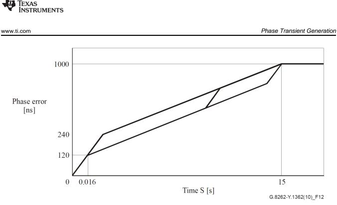
Figure 24. Maximum Phase Transient at the Output Due to Reference Switching for EEC-Option 1
