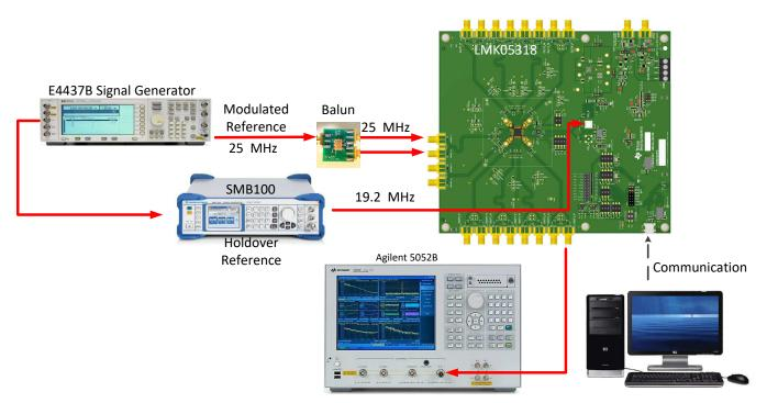
Figure 20. Test Setup for Jitter Tolerance
