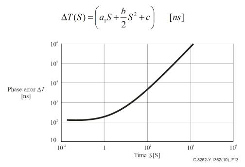
Figure 33. Permissible Phase Error for an EEC-Option 1 Under Holdover Operation at Constant Temperature
