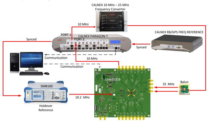
Figure 16. Test Setup for Wander Tolerance
