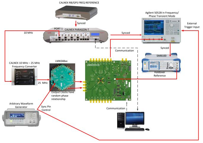
Figure 36. Alternate Test Setup to Measure Phase Transient Response Accurately
