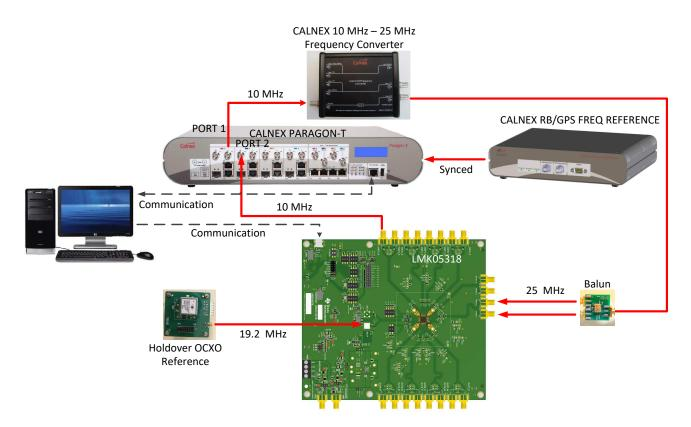
Figure 1. Test Setup for Wander Generation
