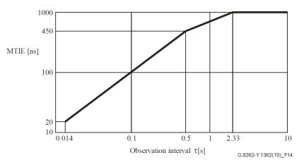
Figure 26. MTIE at the Output Due to Reference Switching/Rearrangement Operations for EEC-Option 2
