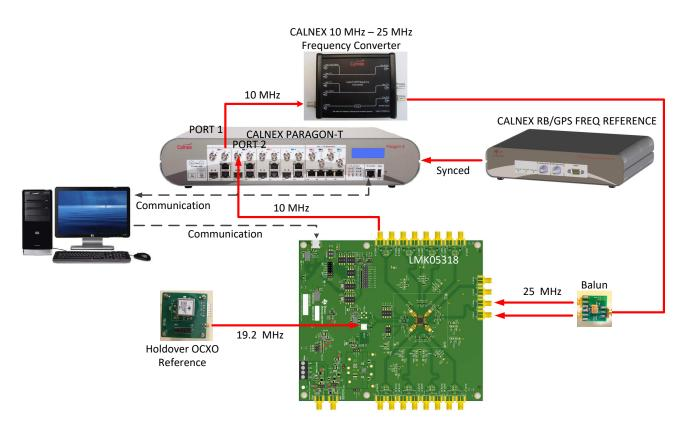
Figure 11. Test Setup for Wander Transfer
