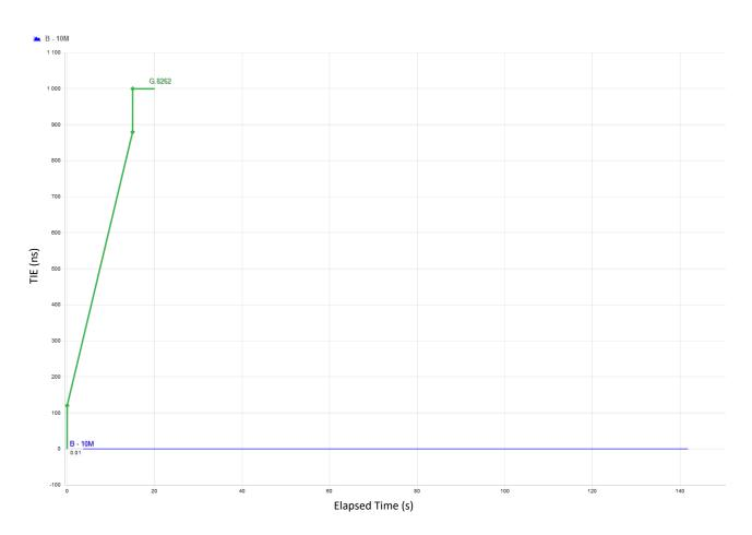
Figure 29. Phase Transient With Signal Interruptions Results
