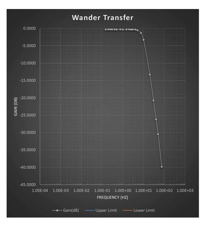
Figure 12. Wander Transfer EEC Option 1 With Max DPLL Bandwidth of 10 Hz
