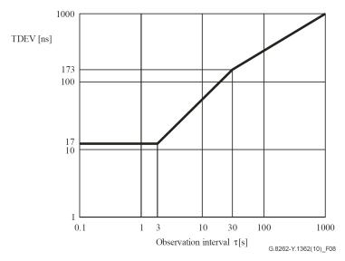
Figure 14. Input Wander Tolerance (TDEV) for EEC-Option 2
