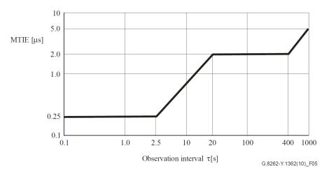
Figure 17. Input Wander Tolerance (MTIE) for EEC-Option 1
