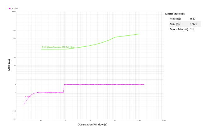
Figure 4. Wander Generation MTIE Option 1, G.8262 EEC Option 1 Results, Tested at Temperature of 85°C With DPLL Bandwidth of 10 Hz
