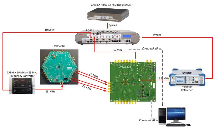
Figure 23. Test Setup for Phase Transient Generation
