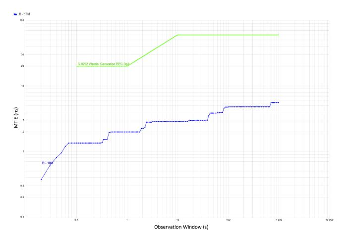
Figure 8. Wander Generation MTIE ITU-T G.8262 EEC Option 2 Results, Tested at Constant Room Temperature With DPLL Bandwidth of 0.1 Hz
