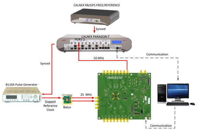
Figure 28. Test Setup for Phase Transient Generation With Signal Interruption
