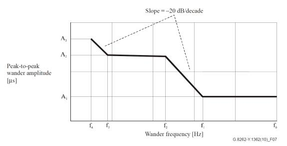
Figure 18. Lower Limit of Maximum Tolerable Sinusoidal Input Wander for EEC-Option 1
