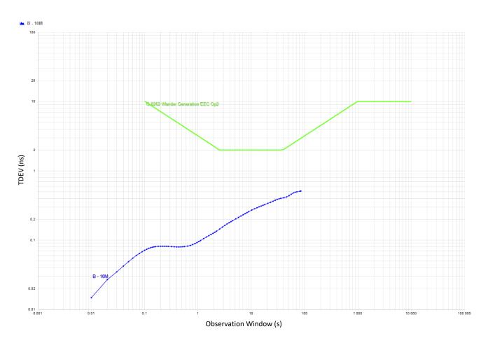
Figure 10. Wander Generation TDEV G.8262 EEC Option 2 Results, Tested at Constant Room Temperature With DPLL Bandwidth of 0.1 Hz
