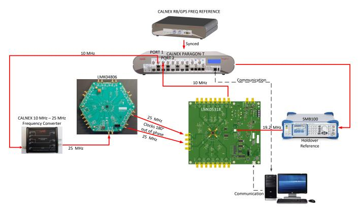
Figure 30. Test Setup for Phase Discontinuity
