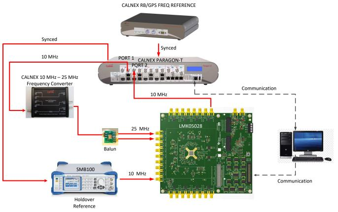
Figure 16. Test Setup for Wander Tolerance
