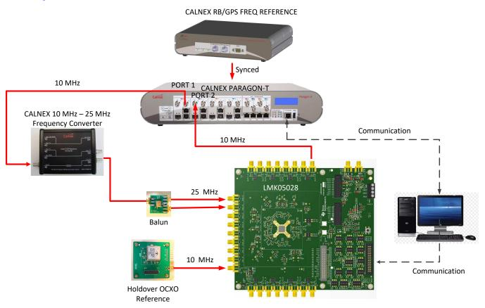
Figure 11. Test Setup for Wander Transfer
