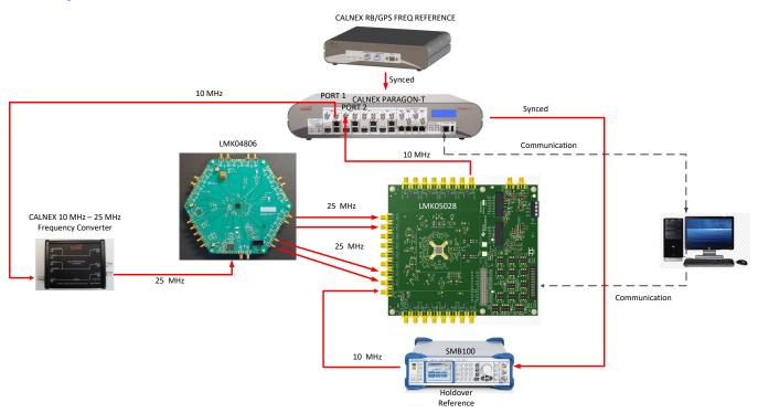
Figure 23. Test Setup for Phase Transient Generation
