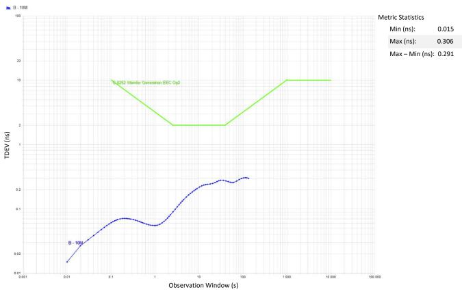
Figure 10. Wander Generation TDEV G.8262 EEC Option 2 Results, Tested at Constant Room Temperature With DPLL Bandwidth of 0.1 Hz
