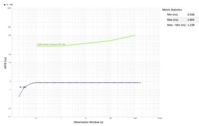
Figure 3. Wander Generation MTIE Option 1, G.8262 EEC Option 1 Results, Tested at Constant Room Temperature With DPLL Bandwidth of 10 Hz
