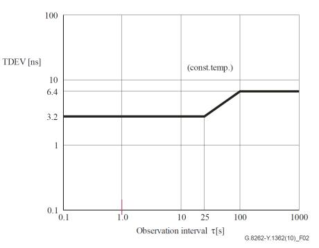
Figure 5. Wander Generation (TDEV) for EEC-Option 1 With Constant Temperature
