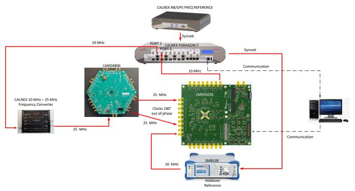
Figure 30. Test Setup for Phase Discontinuity
