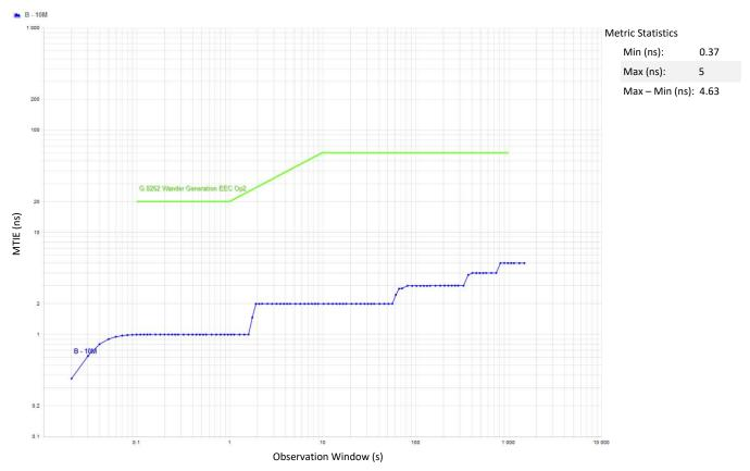
Figure 8. Wander Generation MTIE ITU-T G.8262 EEC Option 2 Results, Tested at Constant Room Temperature With DPLL Bandwidth of 0.1 Hz
