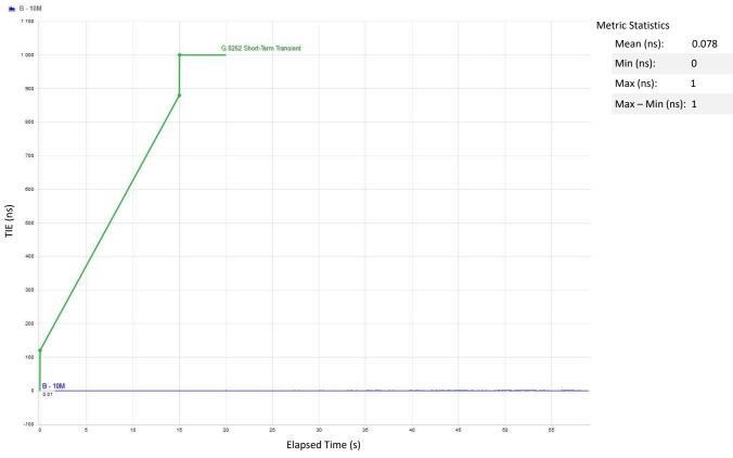
Figure 25. Short-Term Phase Transient Result
