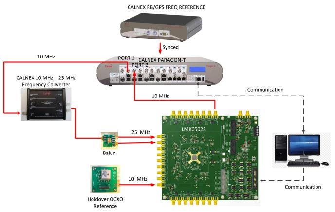
Figure 1. Test Setup for Wander Generation
