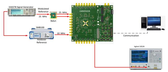
Figure 20. Test Setup for Jitter Tolerance
