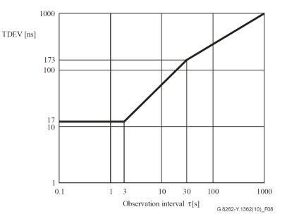
Figure 14. Input Wander Tolerance (TDEV) for EEC-Option 2
