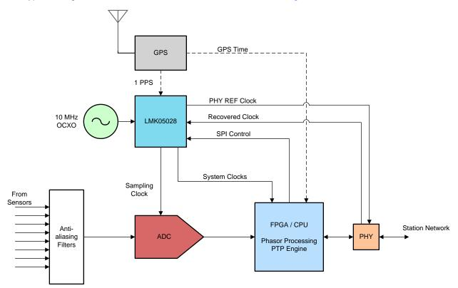
A typical usage of LMK05028 in a Smart Grid PMU is shown in Figure 16 below.
