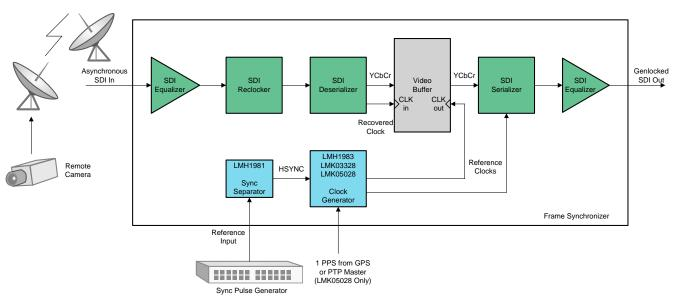
Figure 18. LMK05028 in Frame Synchronizer
