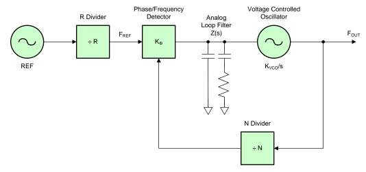
Figure 1. The Basic Analog PLL
