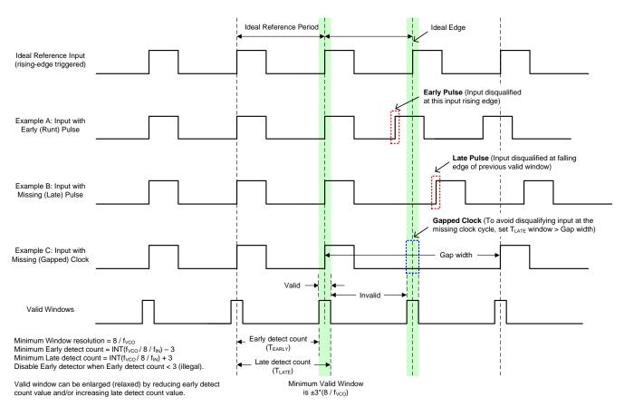
Figure 10. Window Detector Implementation in LMK05028
