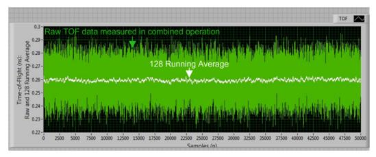
Figure 12. TDC7201 Combined Measurement Data for TOF=0.25ns: Raw and 128x Running Average
