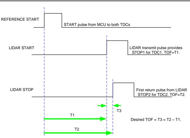
Figure 6. TDC7201 Short Time Measurements Timing Diagram
