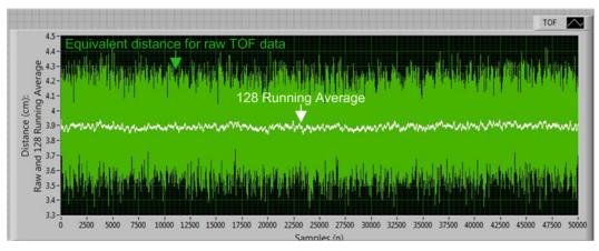
Figure 13. TDC7201 Combined Measurement Data for TOF=0.25ns: Equivalent Distance Raw and 128x Running Average
