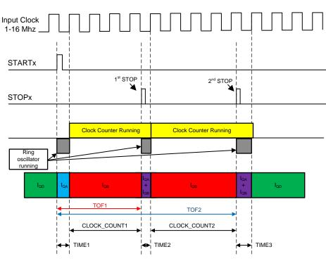
Figure 4. TDCx Measurement Mode 2
