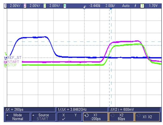
Figure 8. DTG5078 Generated Test Signals For Interleaved Short Time Measurements
