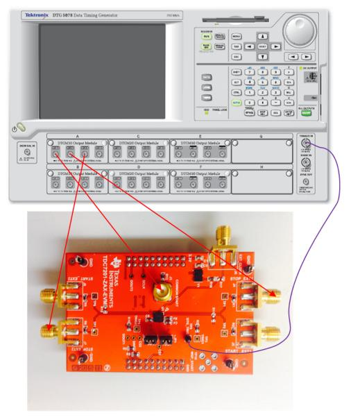
Figure 7. DTG5078 Based Test Setup
