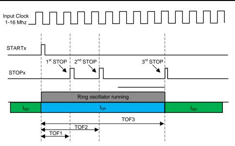
Figure 3. TDCx Measurement Mode 1
