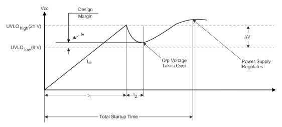
Figure 4. Timing Diagram of Startup Sequence in UCC28722
