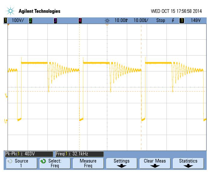
Figure 12. SW Node Waveform at  $V_{\rm IN}$  = 230  $V_{\rm AC}$  for a 8 W Bulb
