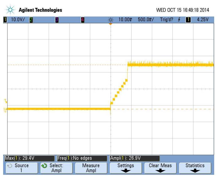
Figure 18.  $V_{OUT}$  Turn on Waveform at  $V_{IN}$  = 230  $V_{AC}$  for a 5 W LED Bulb
