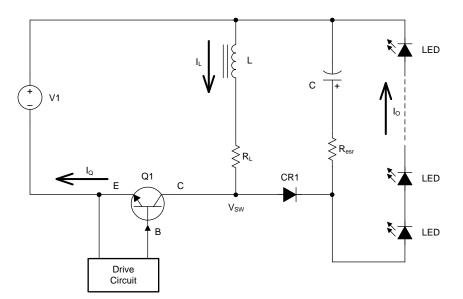
Figure 1. Buck-Boost Power Stage Schematic
