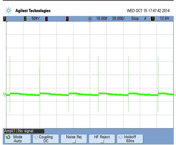
Figure 15.  $V_{OUT}$  Ripple at  $V_{IN}$  = 230  $V_{AC}$  for a 7 W Bulb
