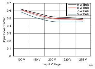
Figure 9. Input Power Factor vs V<sub>IN</sub>
