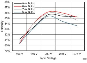
Figure 6. Efficiency vs V<sub>IN</sub>
