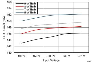
Figure 7. Line Regulation vs V<sub>IN</sub>
