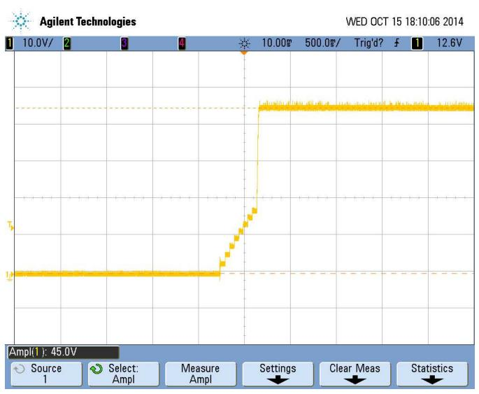
Figure 20.  $V_{OUT}$  Turn on waveform at  $V_{IN}$  =230  $V_{AC}$  for a 8 W LED Bulb
