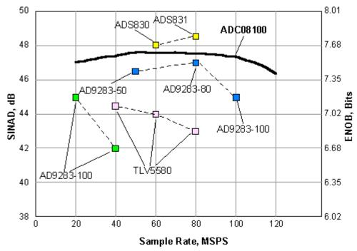
Figure 2. The ADC08100 provides a flatter performance response
