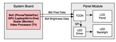
Figure 3. GPU-led HDR display architecture.
