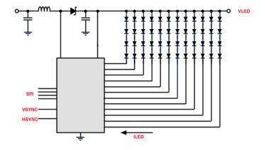
refresh them fast enough so that the transitions are seamless to the human eye. As you may imagine, the communication interface has to be significantly faster. Typically, you may see a +10MHz Serial Peripheral Interface (SPI) or similar protocol on an HDR backlight driver.
