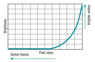
*Figure 2.* Extended Society of Motion Picture and Television Engineers (SMPTE) ST2084 EOTF.
