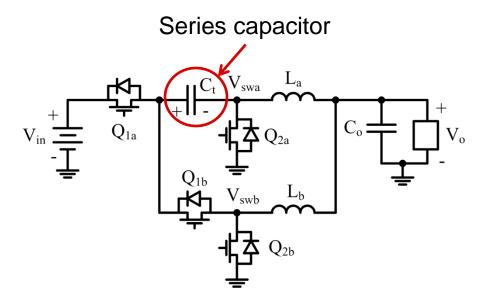
Two-phase, series cap buck converter
