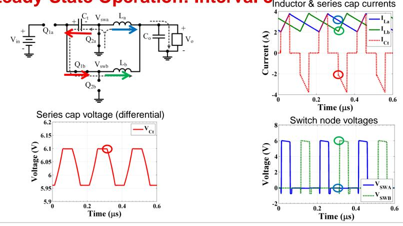
Steady-State Operation: Interval 3<sub>Inductor & series cap currents</sub>
