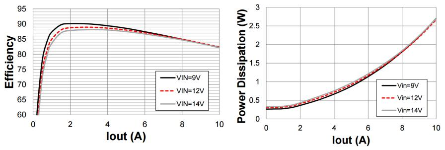
Over 90% efficiency at 9 V input, less than 3 W loss at full load
