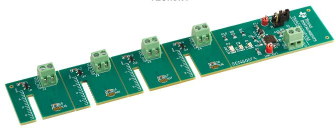
This user's guide describes the characteristics, operation, and use of the TMAG5124 2-wire evaluation module (EVM). This EVM is designed to evaluate the performance of the TMAG5124 over a separation of distance using current as the signal of interest. This document includes a schematic, printed-circuit board (PCB) layouts, and a complete bill of materials (BOM).
