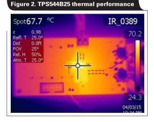
input and 1.2-V output at 20 A. Conditions for the TPS544B25 were a 12-V input and 0.95-V output at 20 A. The TPS40400 controller solution reached a maximum temperature of 47°C, while the TPS544B25 converter reached a maximum temperature of 67.7°C. These images show that spacing the MOSFETs away from the controller can enable better thermal performance and reduce the risk of causing failures or permanent damage to the board.
