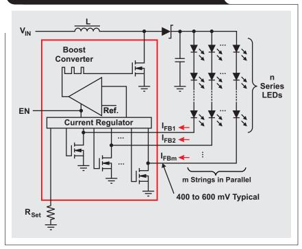
Figure 2. LED driver with integrated current sinks
