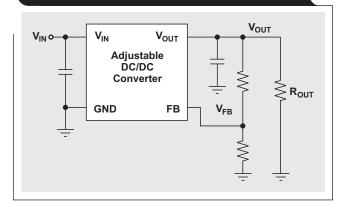
Figure 1. Adjustable DC/DC converter used to
