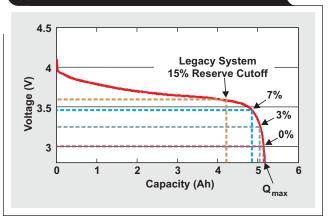
Track system, which can provide up to 99% accuracy, we can program the terminate voltage ( $V_{Term}$ ) at which zero capacity is defined. If we have true 99% accuracy, then the 14% capacity we gain back can be used to significantly increase the run time of the system (see Figure 4).
