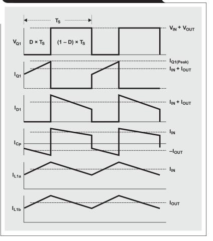
not have equal inductance and the ripple currents will not be exactly equal. Regardless, for a desired ripple-current value, the inductance required in a coupled inductor is estimated to be half of what would be needed if there were two separate inductors, as shown in Equation 4:
