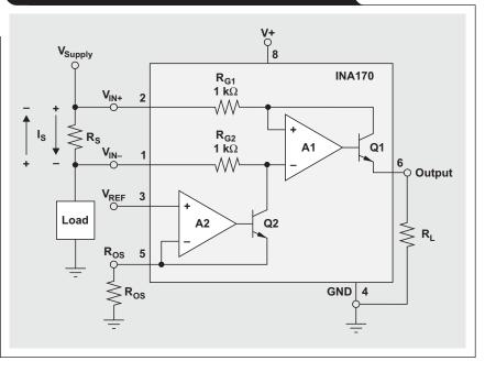
at the same CMV potential; but when a current flows through the shunt resistor, a differential voltage is developed and the inputs become separated by that amount. This voltage difference is amplified by the gain factor of the current-shunt monitor.
