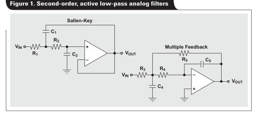
The filter-response DC gain in Figure 2 is equal to 0 dB. The corner frequency of this low-pass filter occurs at 1 kHz, and the gain magnitude at 1 kHz is equal to -3 dB. Following this corner frequency, the filter response falls off at a rate of -40 dB/decade. Theoretically, the attenuation continues to occur as the frequency increases.
