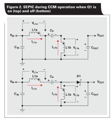
capacitor  $\rm C_P$  is charged to the input voltage,  $\rm V_{IN}.$  Knowing this, we can easily determine the voltages as shown in Figure 3.
