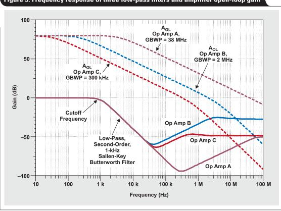
Figure 3. Frequency response of three low-pass filters and amplifier open-loop gain
