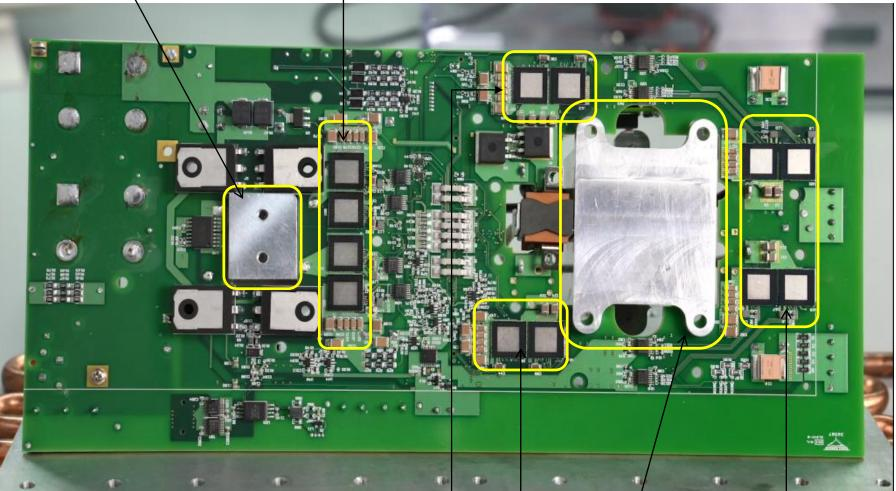
**500-kHz CLLLC transformer** with heatsink
