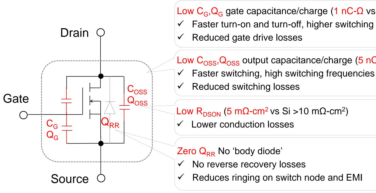
Low  $C_G, Q_G$  gate capacitance/charge (1 nC- $\Omega$  vs Si 4 nC- $\Omega$ ) Faster turn-on and turn-off, higher switching speed
