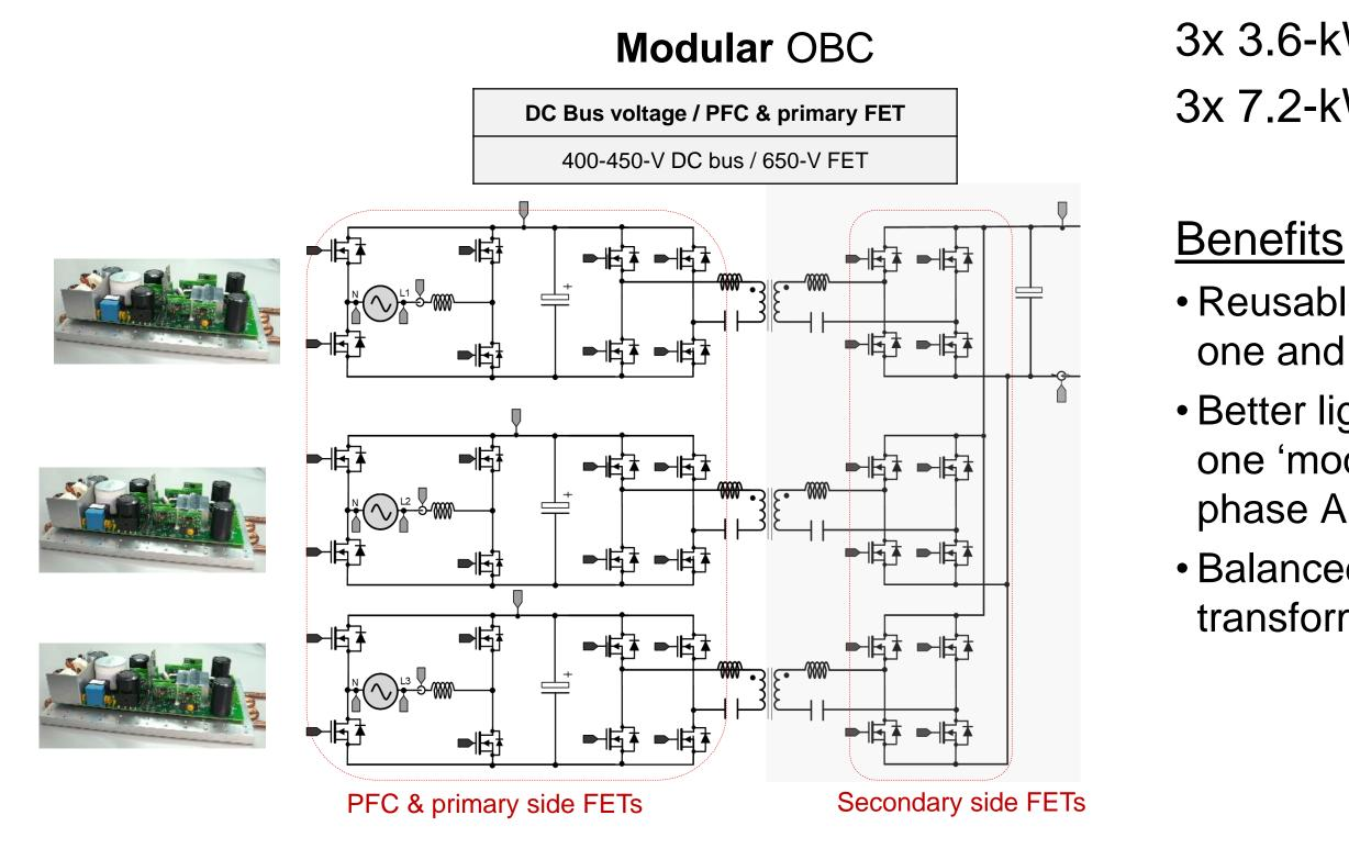
3x 3.6-kW in parallel = 11-kW OBC 3x 7.2-kW in parallel = 22-kW OBC
