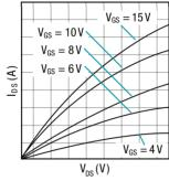
IGBT vs. SiC MOSFET I-V characteristics vary with respect to gate drive voltage (VCC2) and conduction loss
