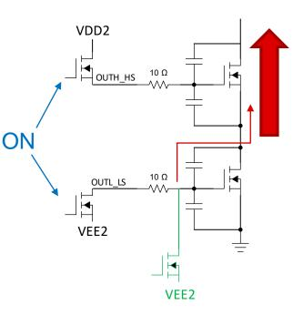
As the SW node rapidly changes, coupling can turn on the External power FETs through the parasitic coupling
