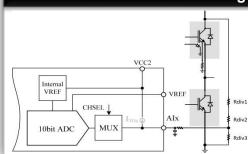
Redundant Bus voltage measurement
