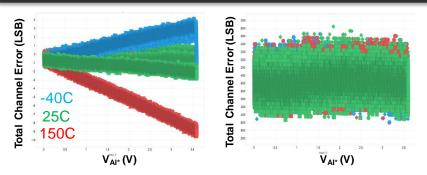
Precision reference can measure AI\* to within +1/-2 LSB (+3.5/-7 mV)
