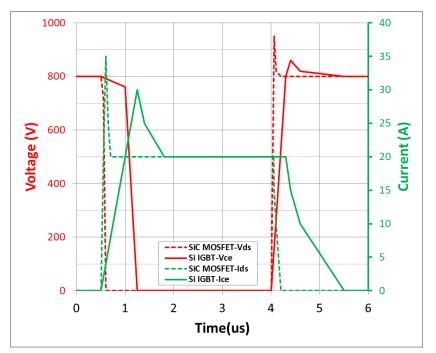
Typical switching waveforms
