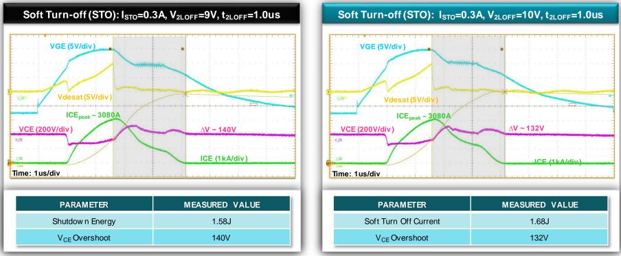
Programmable I<sub>sto</sub> optimizes for the trade-off between shutdown energy and V<sub>CE</sub> overshoot for IGBTs/MOSFETs
