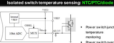
Example using thermal diode + internal VREF
