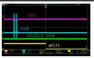
SPI command sent to check VCE Clamp and fault reported showing functioning detection mechanism
