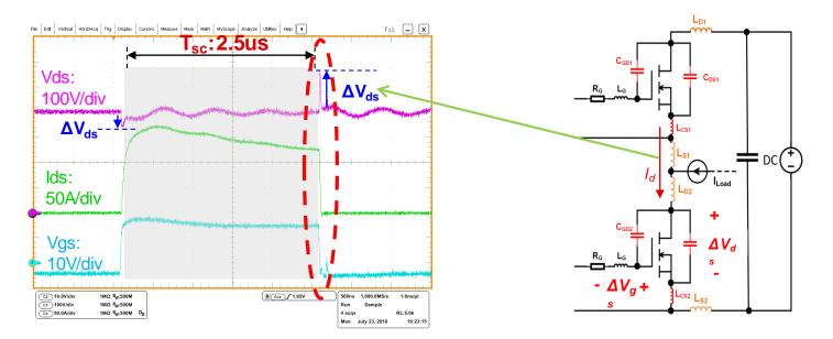
Voltage and avalanche limit: device avalanche can be caused by the overshoot voltage on V<sub>ds</sub>
