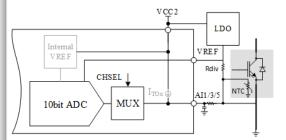
Example using thermal diode + external VREF
