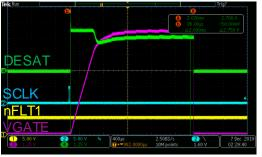
VGTH is accurate measure of health of external power switch Test done with Cree SiC MOSFET C3M0065100K with voltage threshold of 1.8-3V
