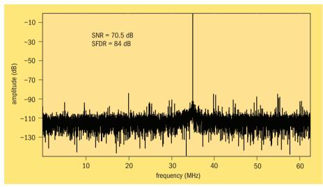
UMTS multicarrier receivers, which must Fig. 2. A fast Fourier transform of a 90 MHz input signal digitized by the ADS5500 sampling at 125 MSPS.
