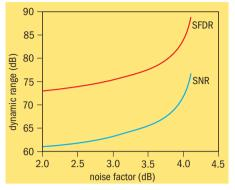
Fig. 3. A plot of the required dynamic performance versus noise factor of a ADS5500-based W-CDMA receiver.
