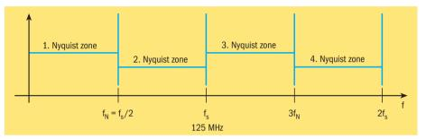
Fig. 1. Texas Instruments' ADC, the ADS5500, has Nyquist zones that are defined by its 125 MSPS sampling rate.
