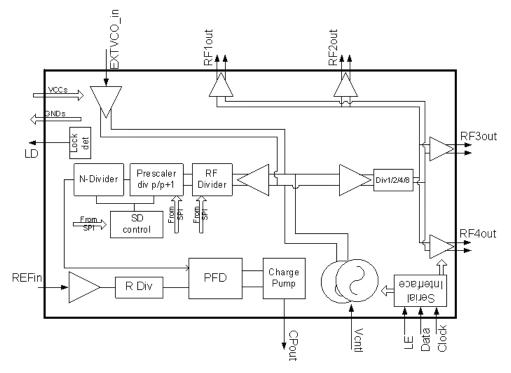
Figure 1. TRF3765 Block Diagram
