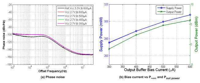
Figure 3. (a) Phase Noise Response at V<sub>cc</sub> 2.7 V for 900 MHz and Different Output Buffer Bias Current Supply. (b) Supply Power and RF Output Power vs Output Buffer Bias Current at 900 MHz and V<sub>cc</sub> 2.7 V
