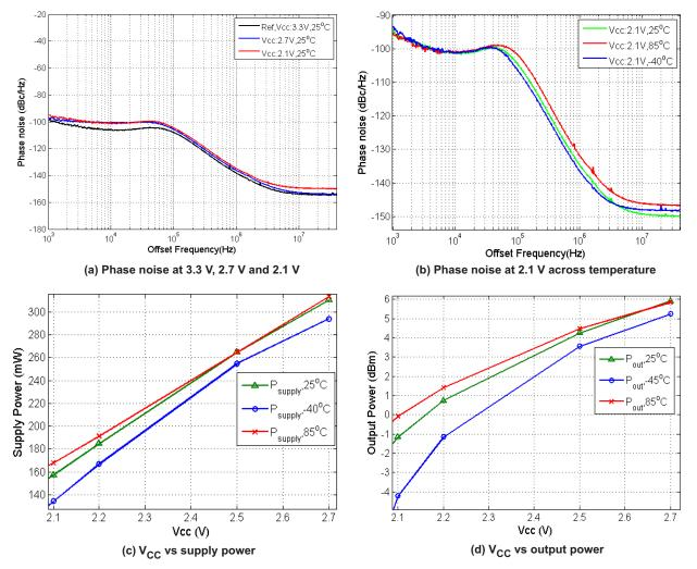
Figure 2. Phase Noise Response for 900 MHz Output, and V<sub>cc</sub> vs Supply and Output Power
