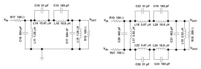
Figure 10. Example of Third-Order Cauer Band-Pass Filter
