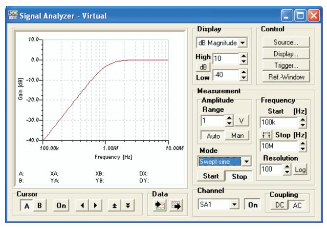
Figure 7. Frequency Response for All Four High-Pass Filters
