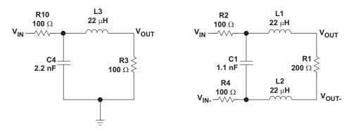
Figure 2. Shunt Capacitor Input Low-Pass Filter
