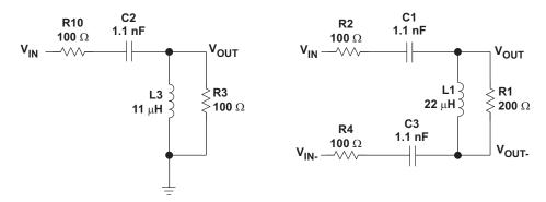
Figure 5. Series Capacitor Input High-Pass Filter
