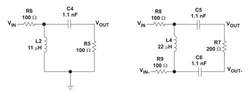
Figure 6. Shunt Inductor High-Pass Filter
