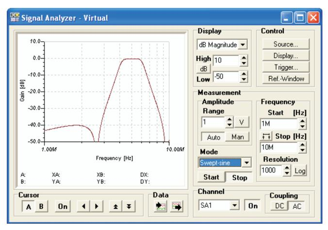
Figure 11. Frequency Response of Third-Order Cauer Band-Pass Filter
