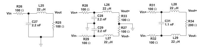
Figure 1. Conversion Process From Single-Ended to a Differential Filter
