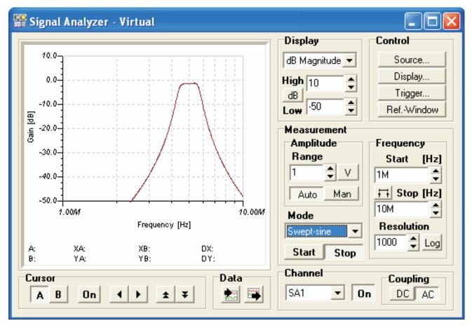
Figure 9. Frequency Response of the Third-Order Butterworth Band-Pass Filter
