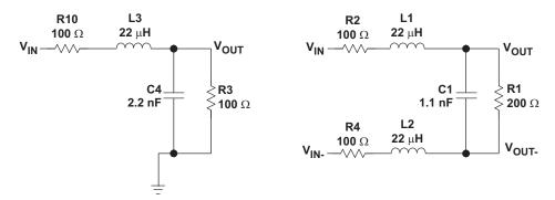
Figure 3. Series Inductor Low-Pass Filter
