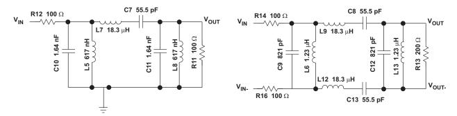
Figure 8. Example of Third-Order Butterworth Band-Pass Filter
