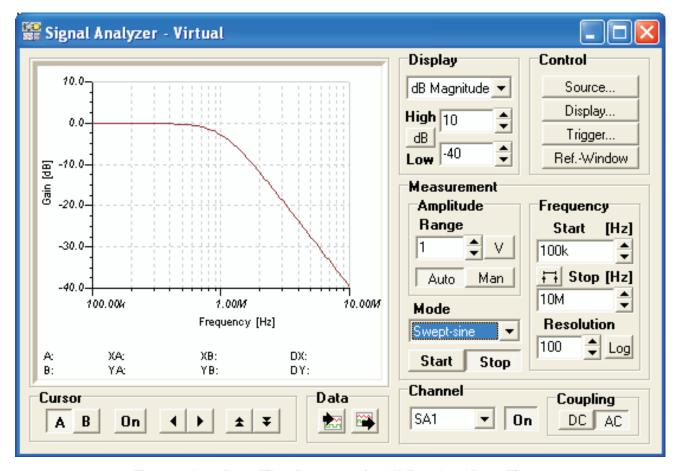
Figure 4. Low-Pass Filter Response for All Four Low-Pass Filters.
