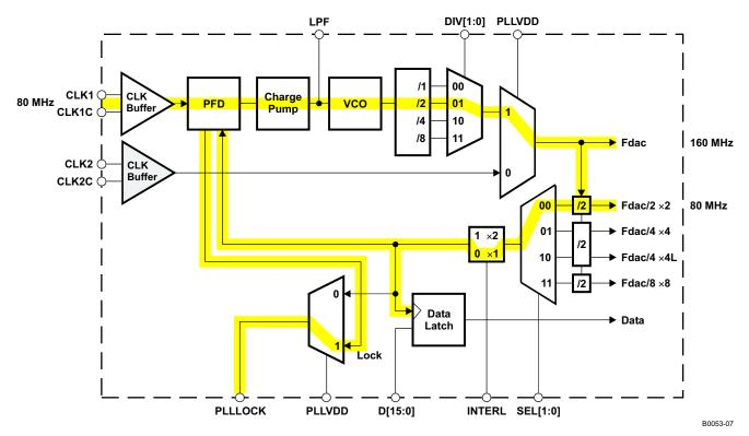
Figure 7. Example 5: Using DIV to Get Different DAC Update Rate
