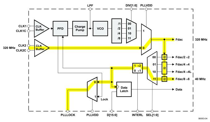
Figure 4. Example 2: External Clock, Interleaved Data
