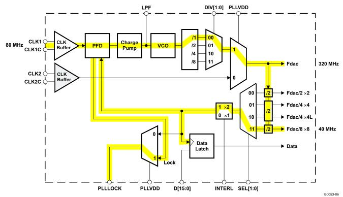
Figure 6. Example 4: PLL Mode With Interleaved Data
