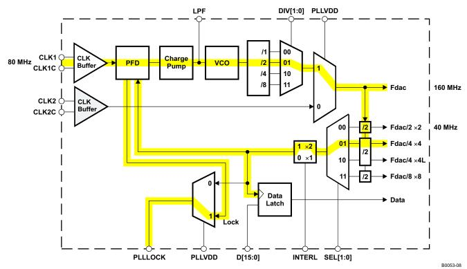
Figure 8. Example 6: Using DIV to Get Different DAC Update Rate With Interleaved Data
