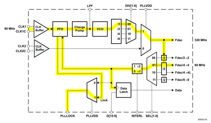
Figure 5. Example 3: PLL Mode Non-Interleaved Data
