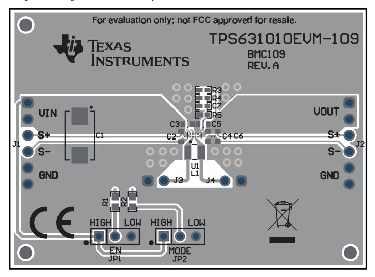
Figure 3-1. Top Layer Routing
