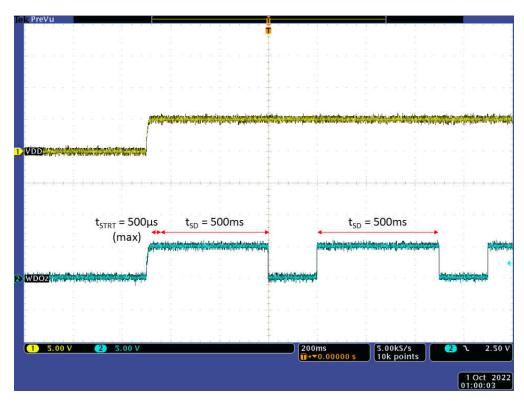
Figure 6-4. Startup Delay
