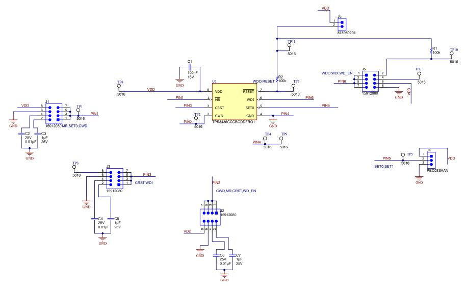
Figure 3-1. TPS36Q1EVM Schematic
