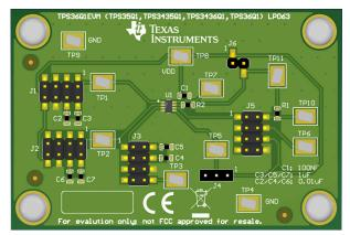
Figure 3-2. Component Placement—Top Assembly
