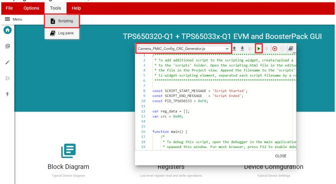
Figure 6-14. GUI Configuration CRC Script
