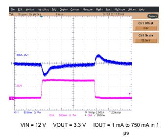
Figure 7-3. Buck 1 Load Transient
