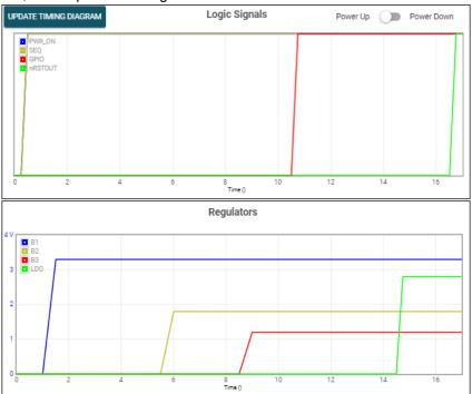
Figure 6-12. GUI Generated Timing Diagram
