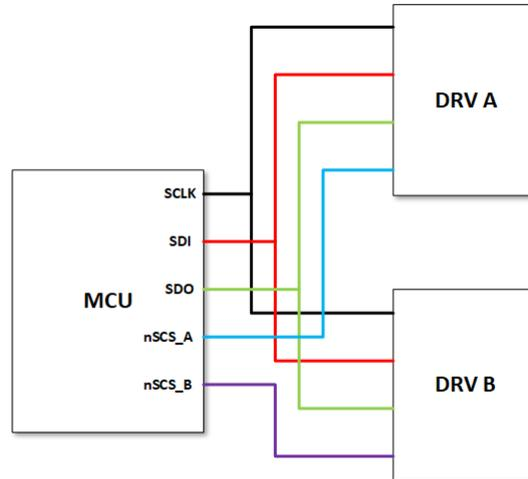
Figure 6-1. Standalone SPI Diagram
