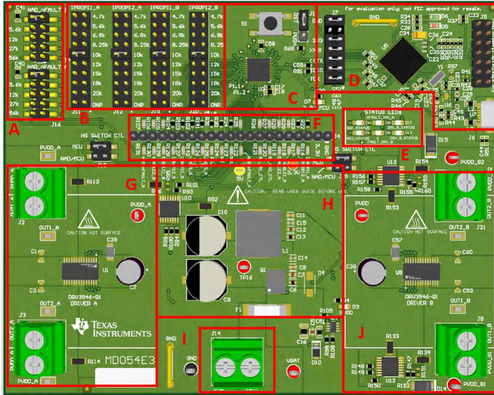
**Figure 2-1. DRV3946-Q1EVM Hardware Components**
