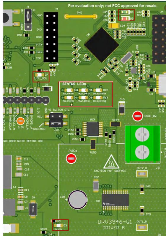
**Figure 2-3. EVM Indicator LEDs**
