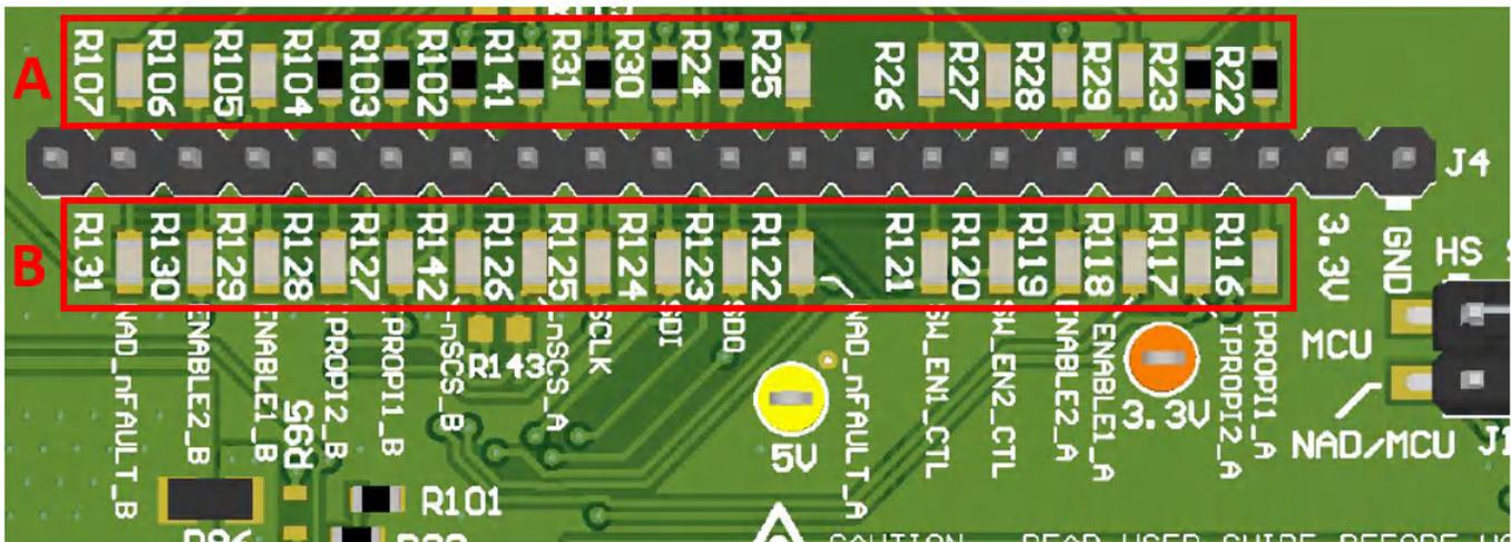
**Figure 2-2. J4 MCU Signal Header**
