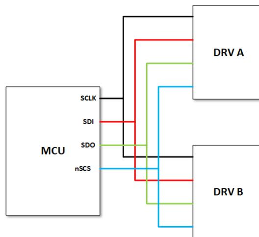
Figure 6-2. Addressable SPI Diagram
