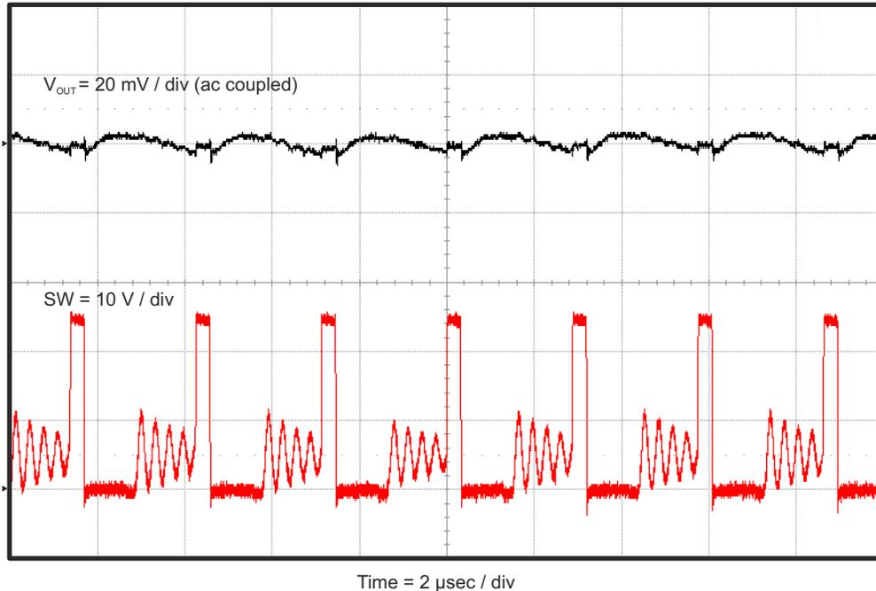
**Figure 2-8. TPS54336AEVM-010 Output Ripple,  $I_{OUT} = 100\text{ mA}$**
