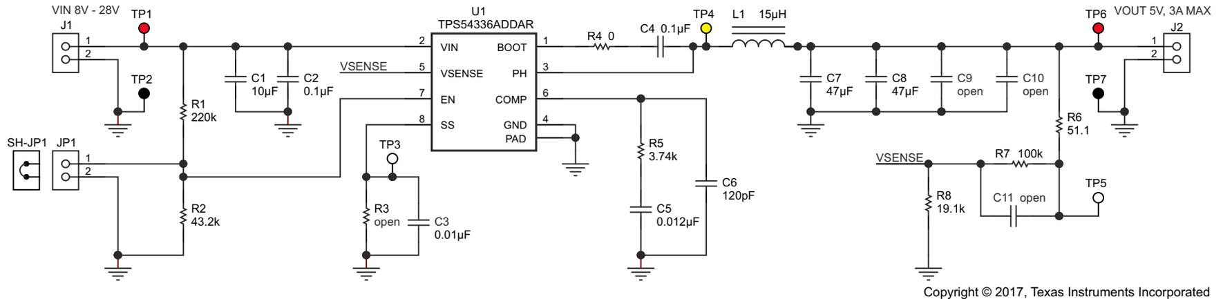
Figure 4-1. TPS54336AEVM-010 Schematic
