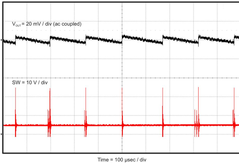
Figure 2-9. TPS54336AEVM-010 Output Ripple,  $I_{OUT} = 0$  A
