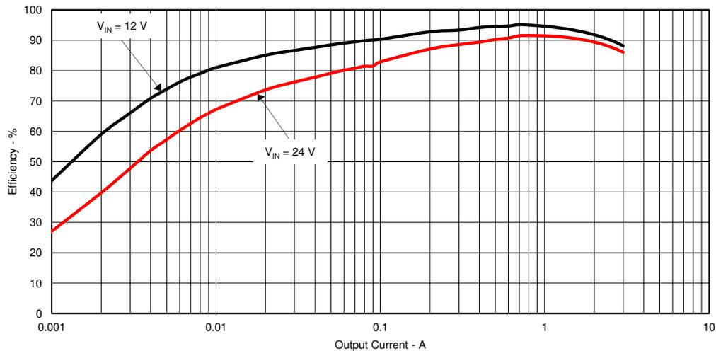
**Figure 2-2. TPS54336AEVM-010 Low Current Efficiency**
