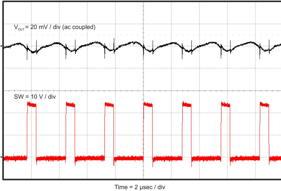
**Figure 2-7. TPS54336AEVM-010 Output Ripple,  $I_{OUT} = 3\text{ A}$**
