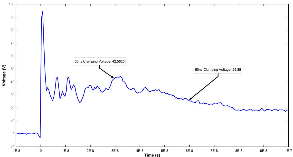
Figure 2. ESD122DMX/DMY 18-kV Contact ESD Strike Waveform
