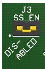
Figure 19. Spread Spectrum Enable Jumper Configuration Default: Jumper Installed, Spread Spectrum Disabled
