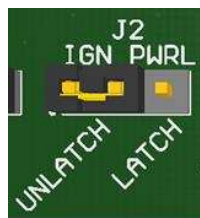
Figure 18. Power-Latch Jumper Configuration Default: LATCH
