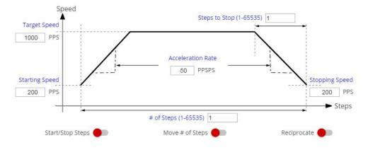
Figure 5. Motor Controls Enabled
