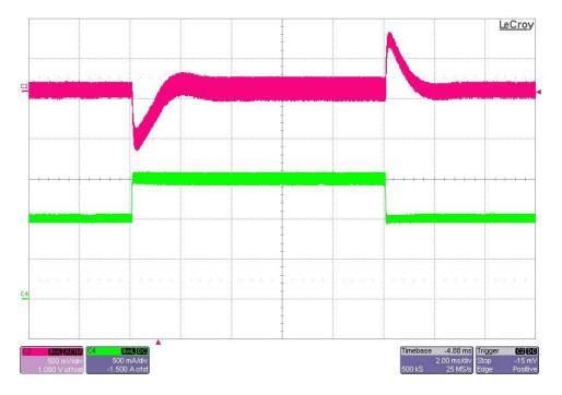
The photo below shows the 15V output voltage (AC coupled) when the load current is stepped from 0.75A to 1.5A. Vin = 4.5Vdc (1V/DIV, 500mA/DIV, 2mS/DIV)
