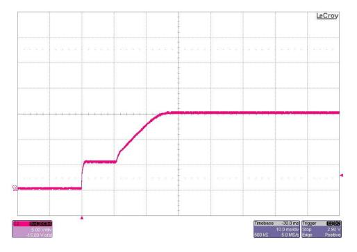
The photo below shows the 15V output voltage startup waveforms after the application of 4.5Vdc in. The output was loaded to 1.5A. (5V/DIV, 10mS/DIV)
