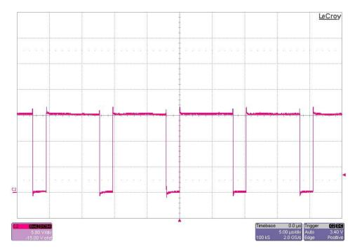
The photo below is the switch-node waveform. The input voltage is 4.5V and the output is loaded to 1.5A. (5V/DIV, 5uS/DIV)
