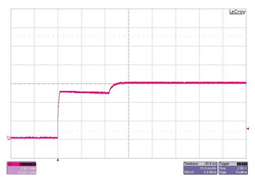
The photo below shows the 15V output voltage startup waveforms after the application of 12Vdc in. The output was loaded to 1.5A. (5V/DIV, 10mS/DIV)
