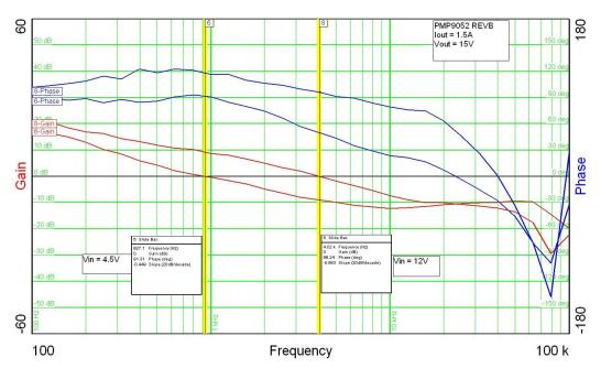
The plot below shows the loop gain with the input voltage at 4.5V and 12V and the output loaded to 0.5A.
