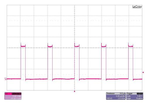
The photo below is the switch-node waveform. The input voltage is 12V and the output is loaded to 0.63A. The converter operates in CCM above this current level. (5V/DIV, 5uS/DIV)
