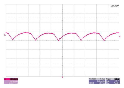
The 15V output ripple voltage (AC coupled) is shown in the figure below. The image was taken with the output loaded to 1.5A and the input voltage set to 4.5Vdc. (100mV/DIV, 5uS/DIV)
