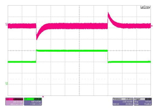
The photo below shows the 15V output voltage (AC coupled) when the load current is stepped from 0.5A to 1.5A. Vin = 12Vdc (500mV/DIV, 500mA/DIV, 2mS/DIV)
