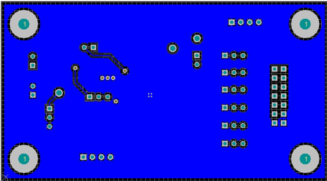
Figure 8. Bottom-Layer Routing
