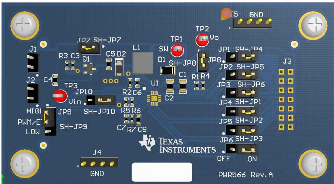
Figure 1. Default Configuration of Jumpers
