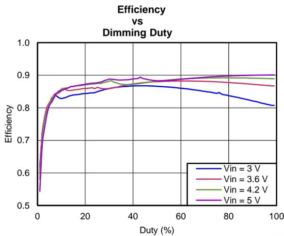
Figure 4. 8s5p, 20 mA/channel
