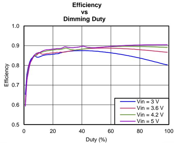
Figure 3. 7s6p, 20 mA/channel
