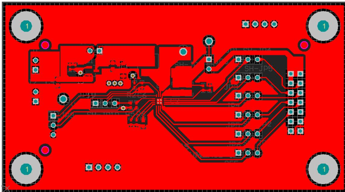
Figure 7. Top-Layer Routing
