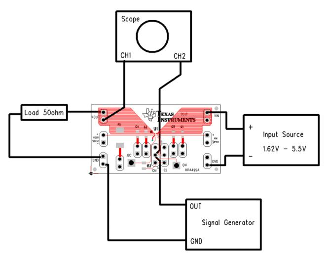
Figure 2. Slew Rate Setup
