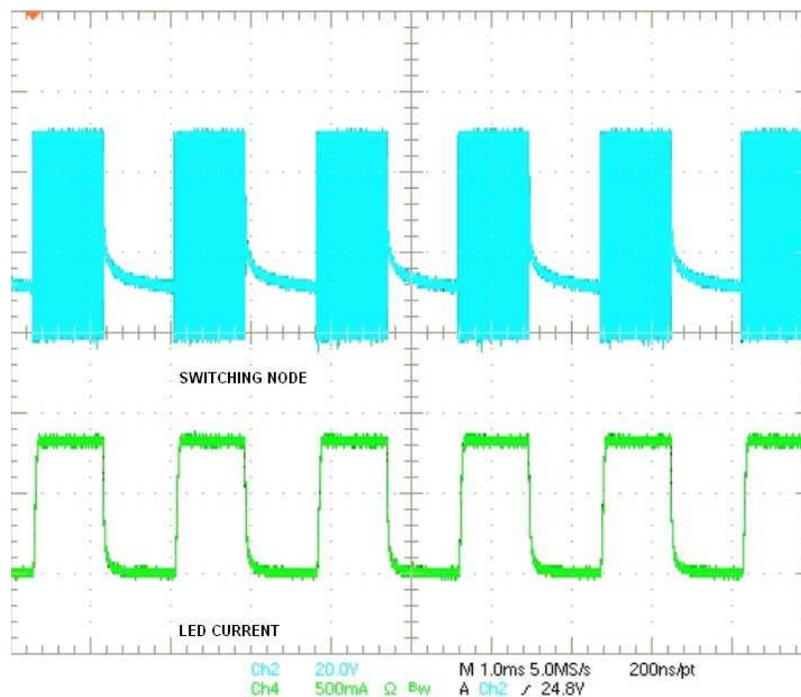
Figure 8. TPS92660EVM Buck Converter PWM Dimming, SADJ = 1.25 V
