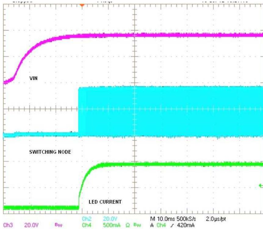
Figure 11. Buck Converter Start-Up Waveform
