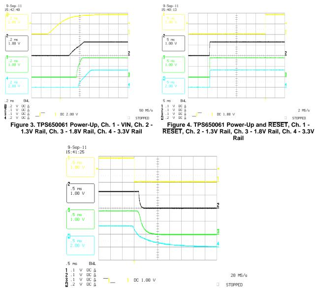
Figure 5. TPS650061 Power-Off Sequence, Ch. 1 - RESET, Ch. 2 - 1.3V Rail, Ch. 3 - 1.8V Rail, Ch. 4 - 3.3V Rail
