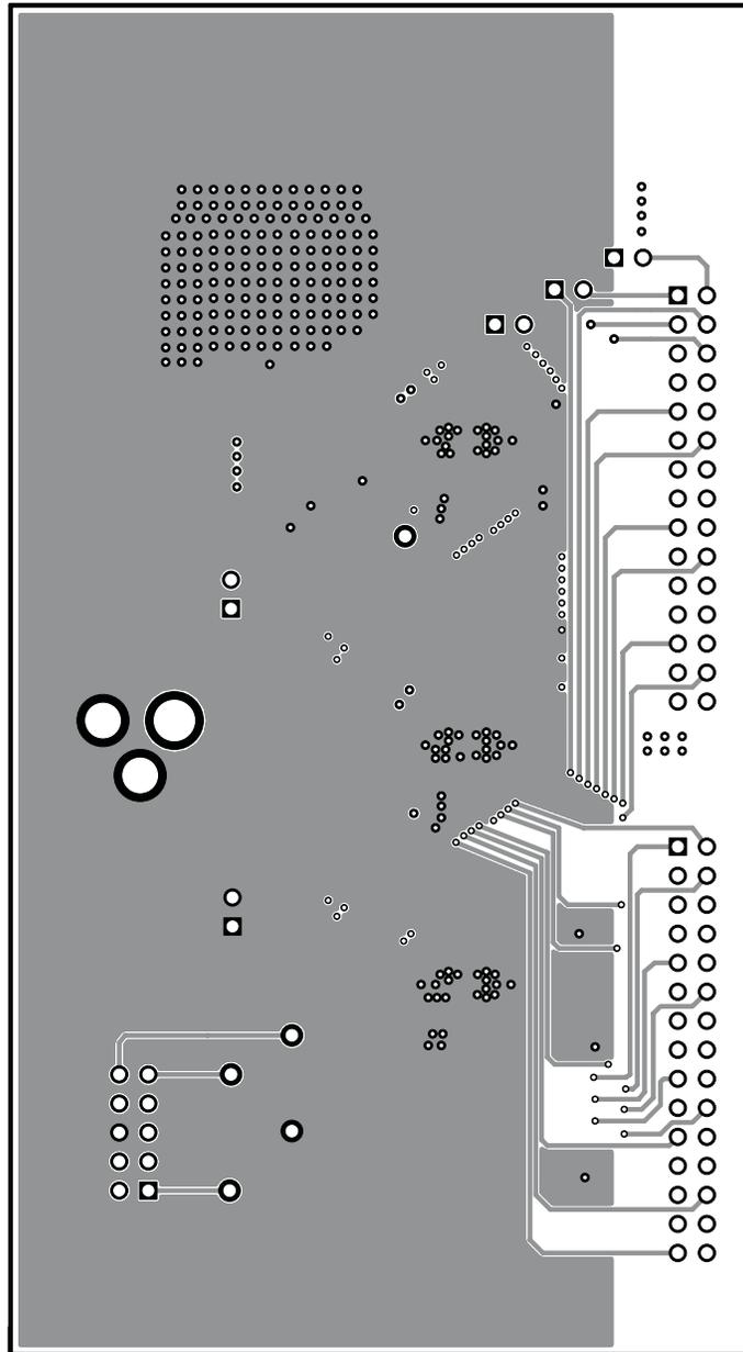
Figure 8. Layer 2 Routing
