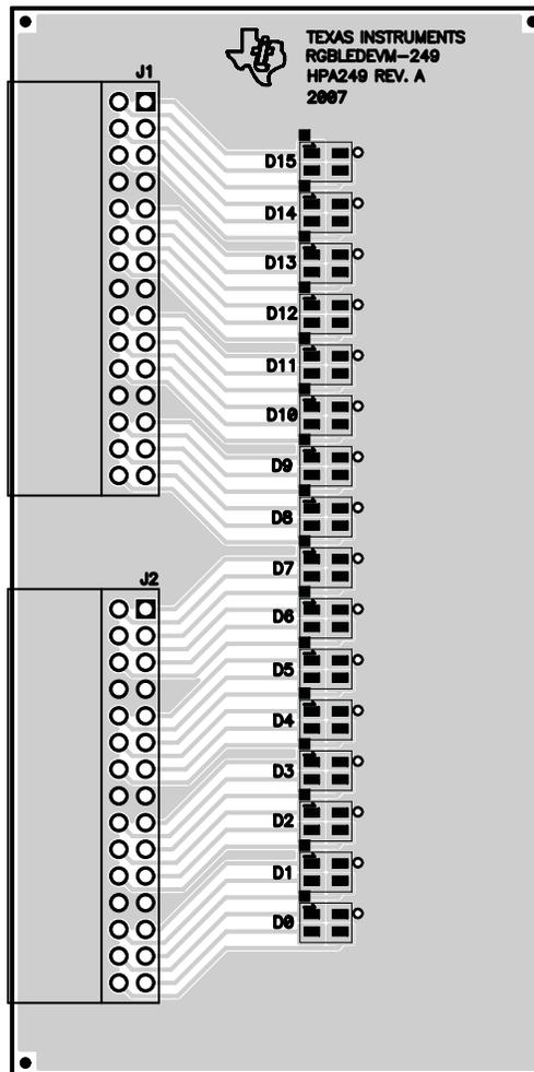
Figure 11. Assembly Layer Routing
