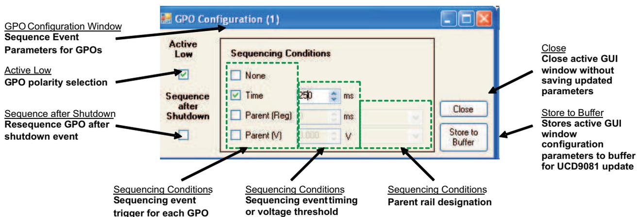
Figure 14. GPO Configuration Option From View Menu Tab
