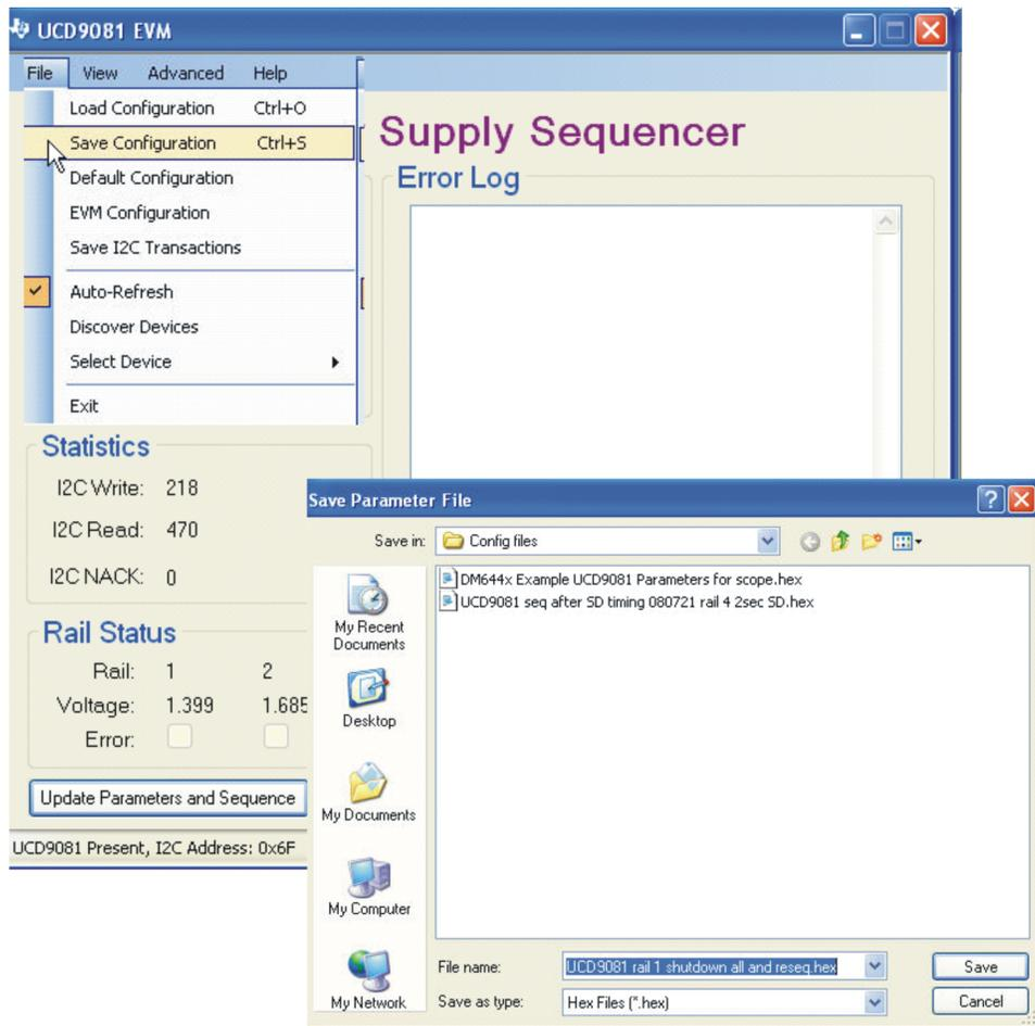
**Figure 4. Save UCD9081 Parameters to Hexadecimal File**
