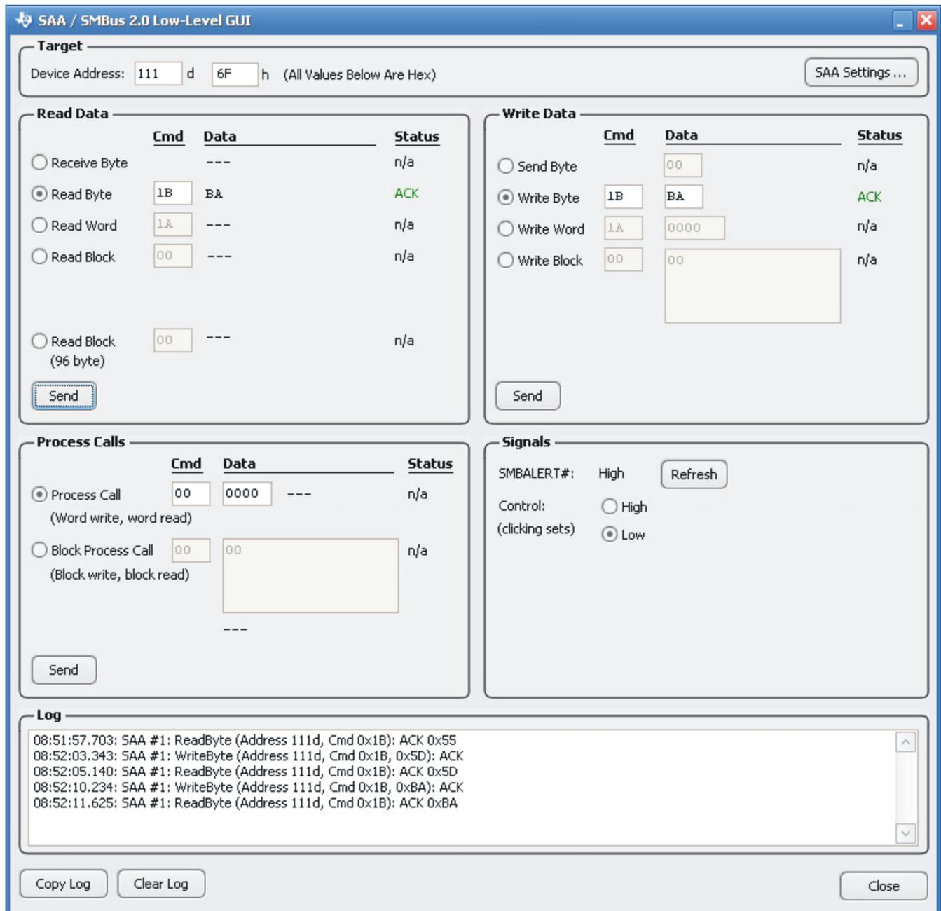
**Figure 30. USB to I<sup>2</sup>C Adapter GUI for Manual Register Reads and Writes**
