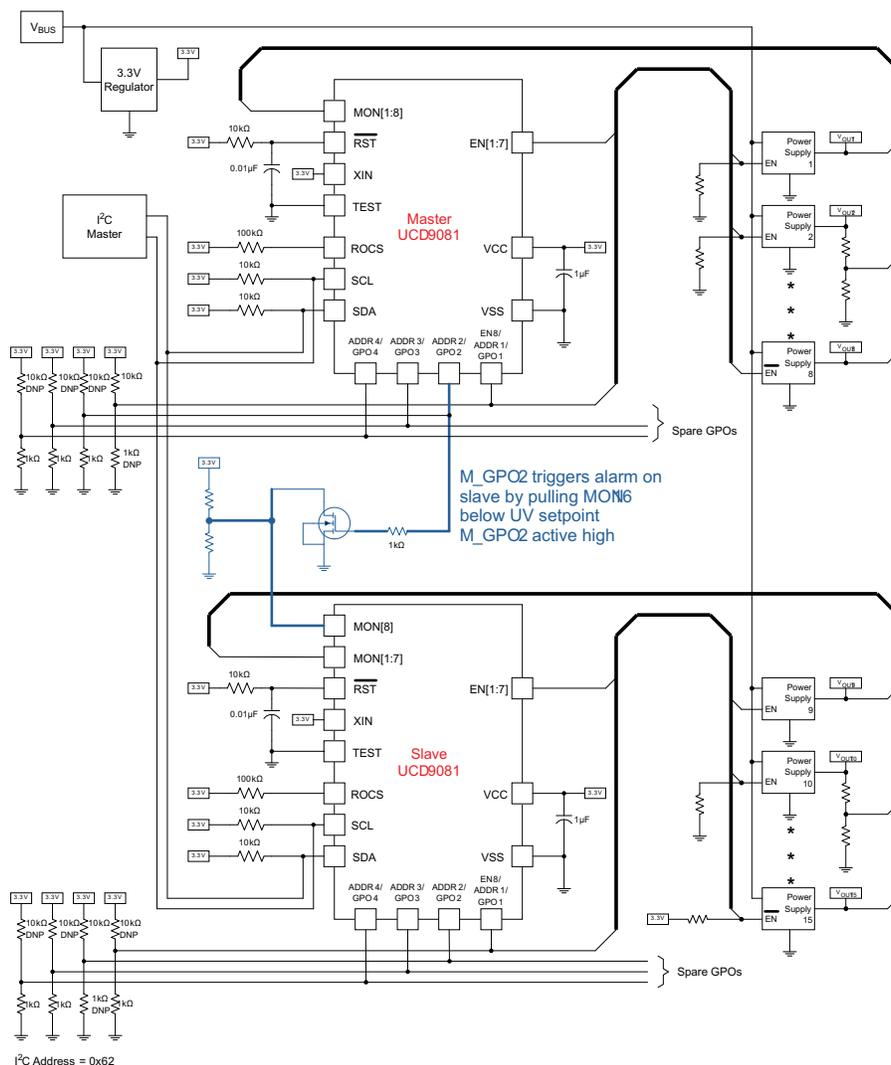
Figure 18. Option for Cascading Multiple UCD9081 ICs
