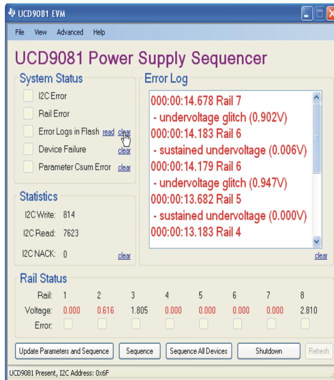
**Figure 2. Clearing Errors Logged in Flash Memory**
