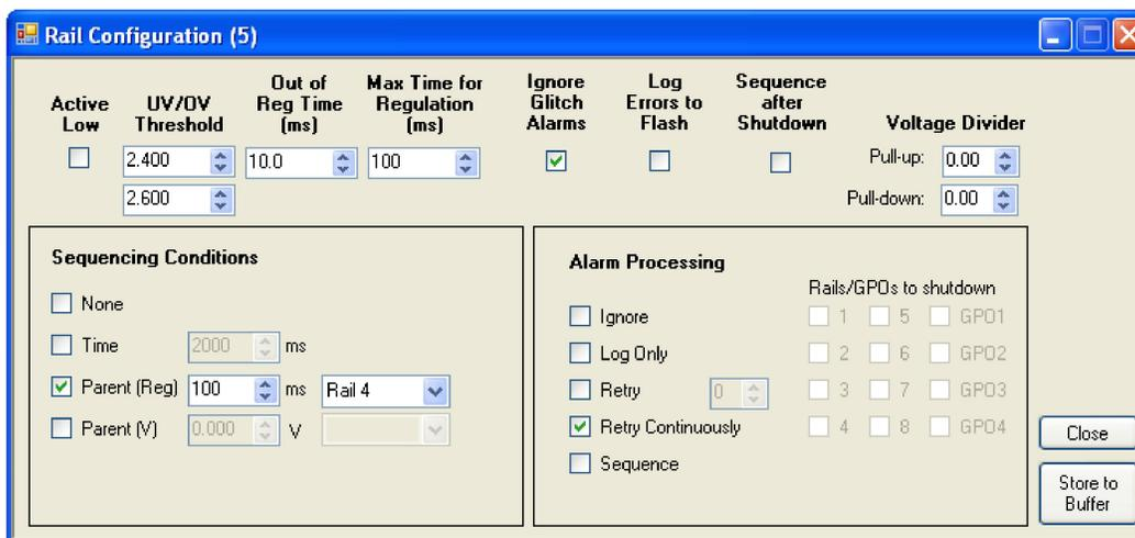
**Figure 27. Example – Configure Rail 5**
