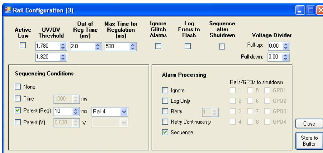
**Figure 25. Example – Configure Rail 3**
