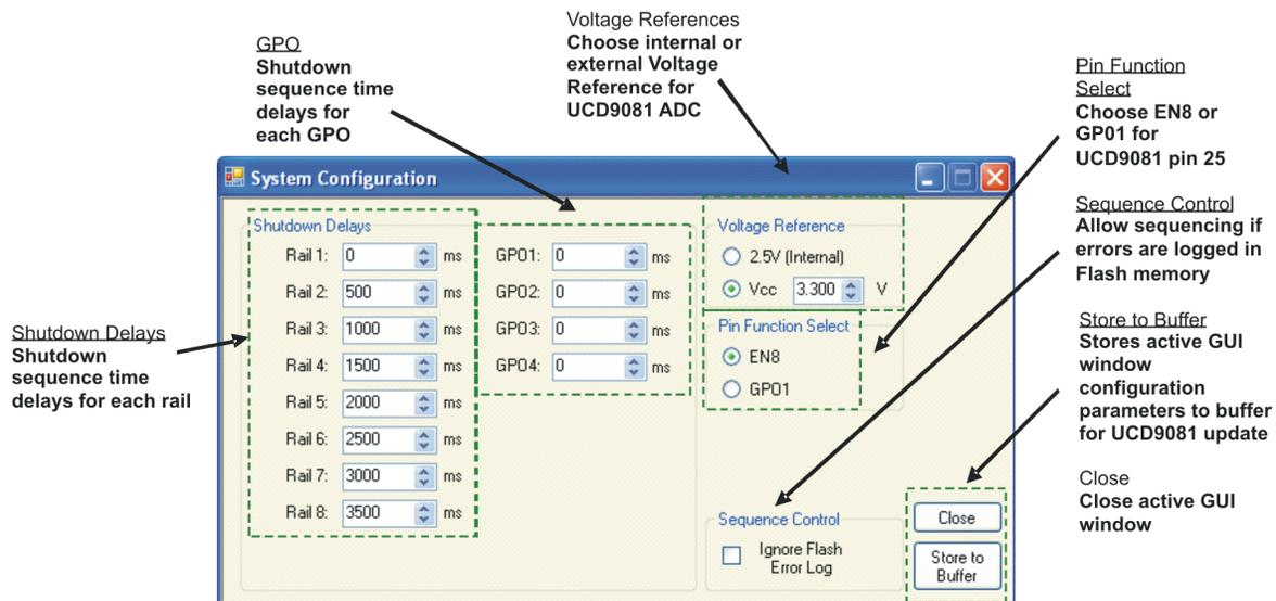
**Figure 7. System Configuration Option From View Menu Tab**
