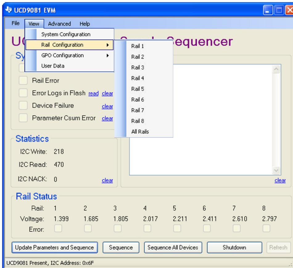
Figure 8. Rail Configuration Drop-Down From View Menu Tab
