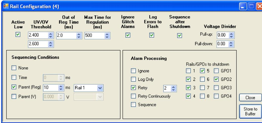
**Figure 26. Example – Configure Rail 4**
