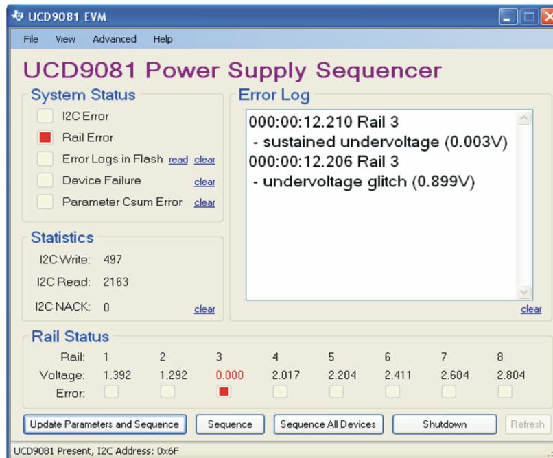
**Figure 1. UCD9081 GUI Main Window**
