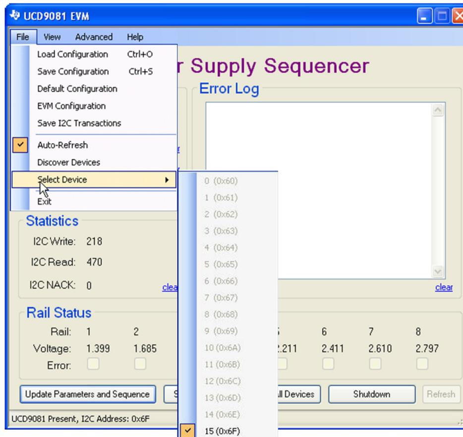
**Figure 5. Select Device Option From File Menu Tab**
