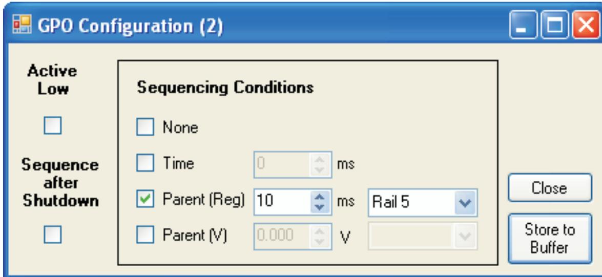
Figure 28. Example – Configure GPO2
