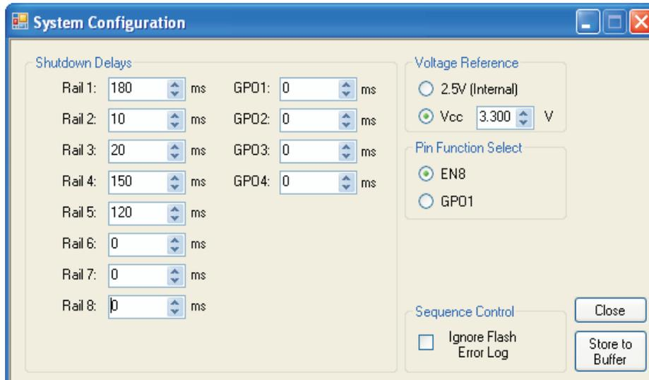
Figure 29. Example – Configure Shutdown Delays for All Rails
