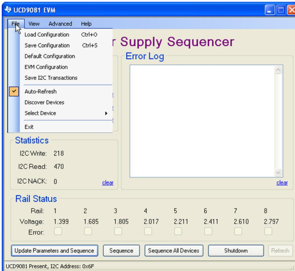
**Figure 3. File Tab From Main Window Menu Bar**
