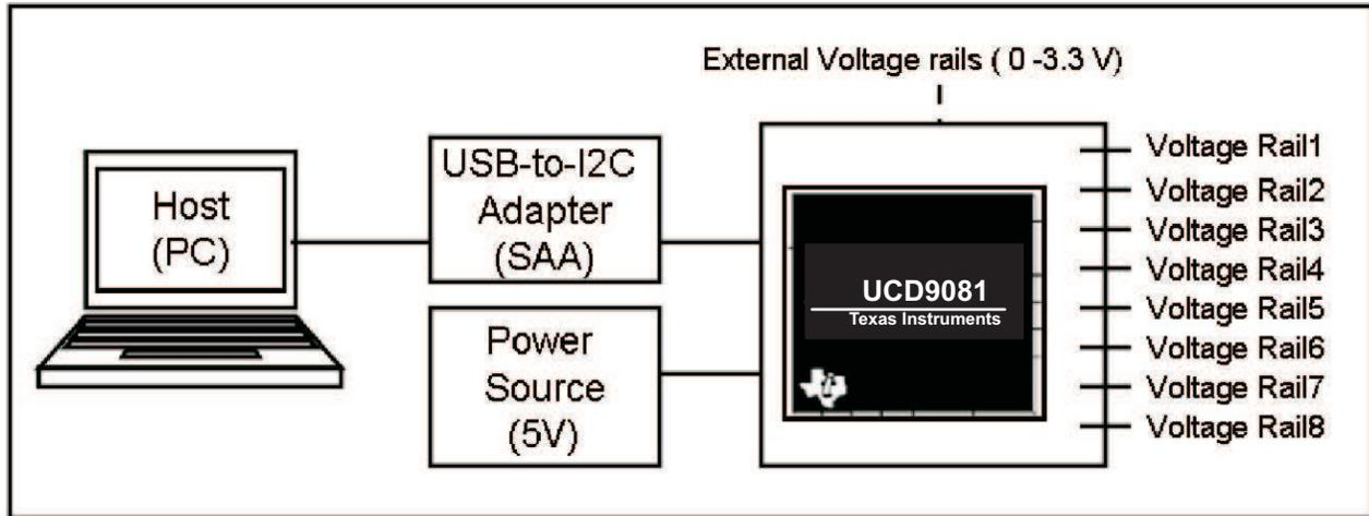
Figure 20. Using the GUI to Communicate With the UCD9081 in a User's Application
