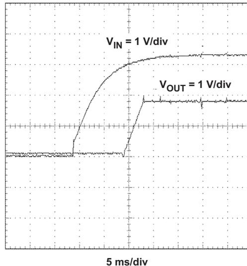
**Figure 8. Power Up, VOUT relative to VIN**
