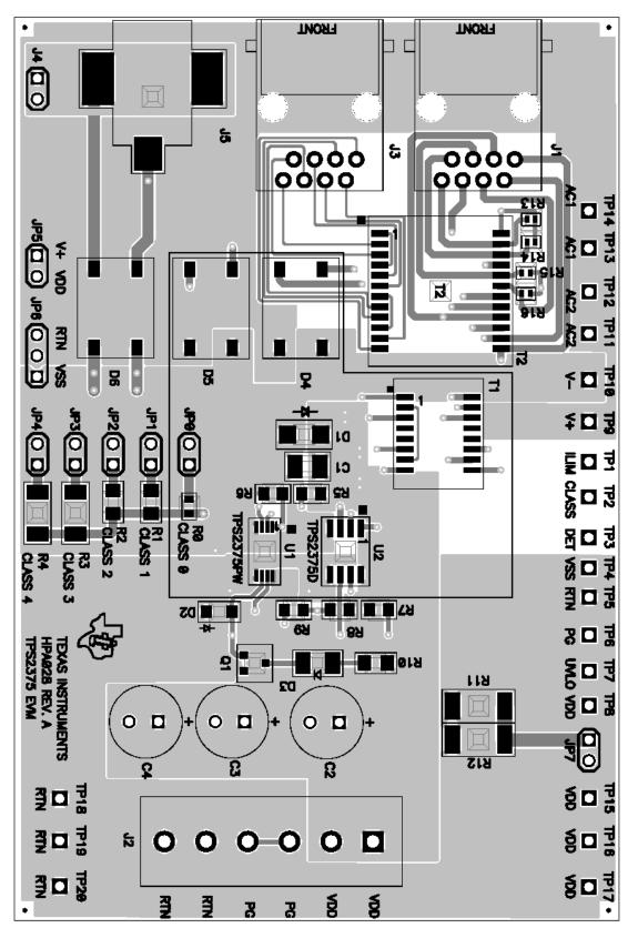
Figure 5–2. Bottom Assembly Layer
