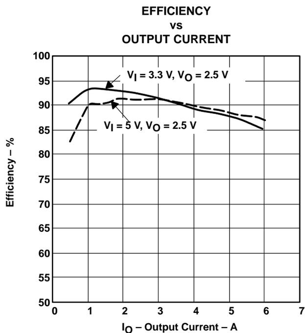
Figure 2–3. Measured Efficiency, TPS54873
