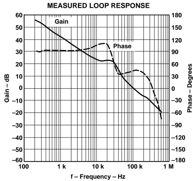
Figure 2–12. Measured Loop Response, TPS54873,  $V_I = 6\text{ V}$
