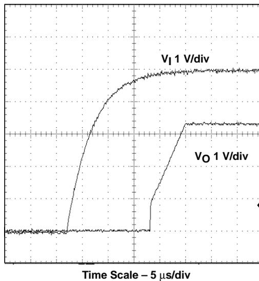
Figure 2–21. Measured Start-Up Waveform, TPS54873 With Precharge
