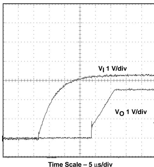
*Figure 2–18* Shows the start-up waveform with the output precharged and a 2- $\Omega$  load. The precharge is achieved by connecting the 3.3-V input to the output with two diodes in series. The start-up mechanism is the same as described above except that the internal reference must ramp up above the voltage fed back from the precharged output to the VSENSE pin before switching can start. Once this occurs, the output continues to ramp up to the output set point of 2.5 V at the slow-start rate.
