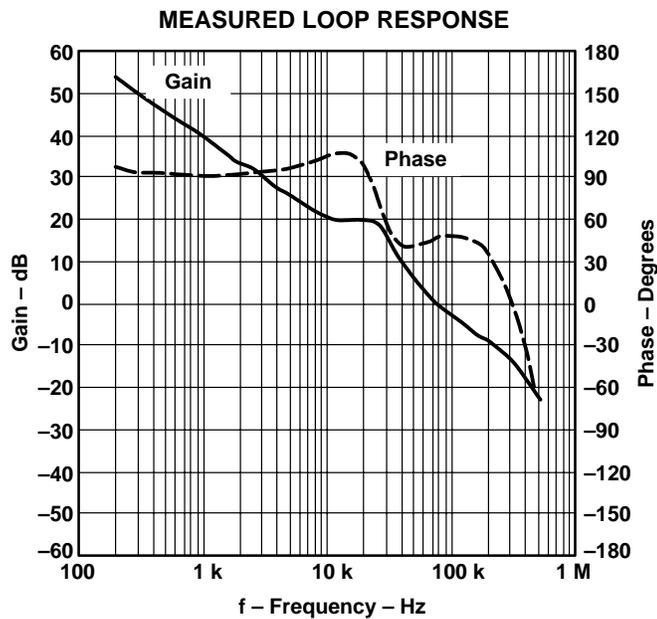
*Figure 2–10. Measured Loop Response, TPS54673,  $V_I = 6\text{ V}$*
