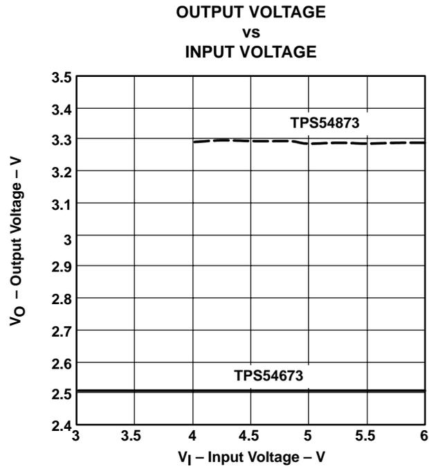
**Note:** The lower limit for the TPS54673 input voltage is about 3.02 V because the device is operating at its maximum duty cycle.
