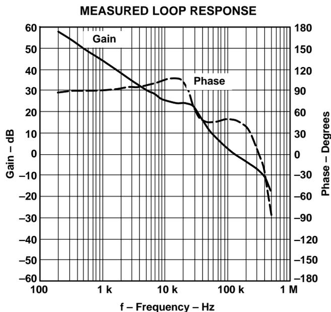
Figure 2–11. Measured Loop Response, TPS54873,  $V_I = 4\text{ V}$
