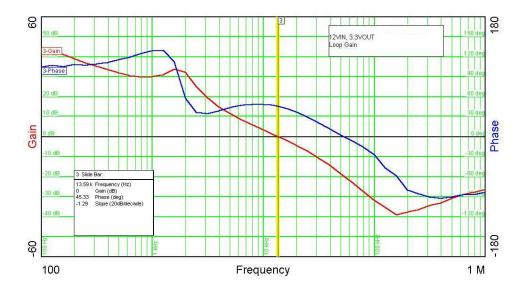
The figure below is the loop gain of the TPS54550 converter with max load. The bandwidth is 20 KHz, the phase margin is 82 degrees, and the gain margin is 28dB.
