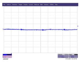
Output ripple/noise 1.2V output:
