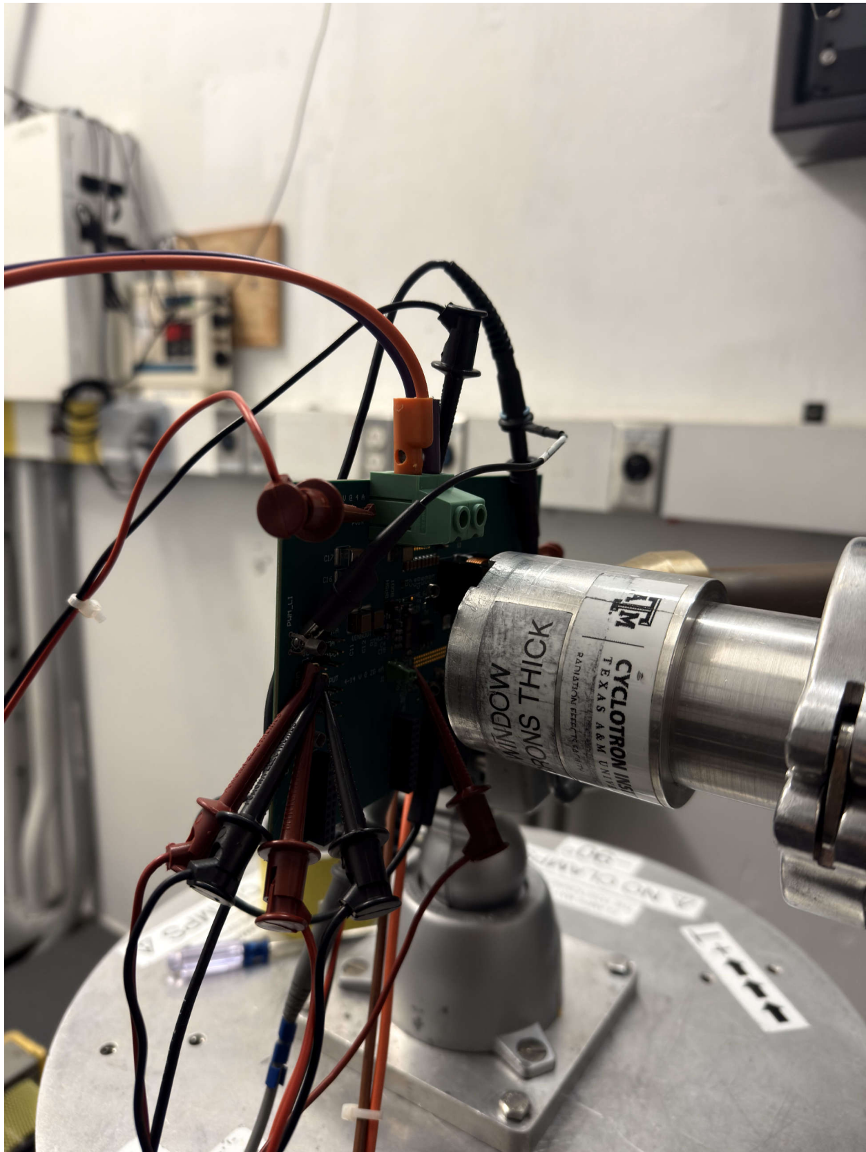
Figure 4-1. TPS7H6101-SEP EVM in Front of the Heavy-Ion Beam Exit Port at the Texas A&M Cyclotron
