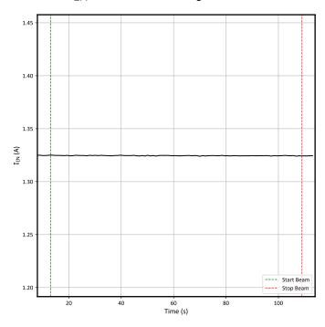
Figure 7-1. Current vs Time for Run # 1 of the TPS7H2221-SEP at T = 125°C
