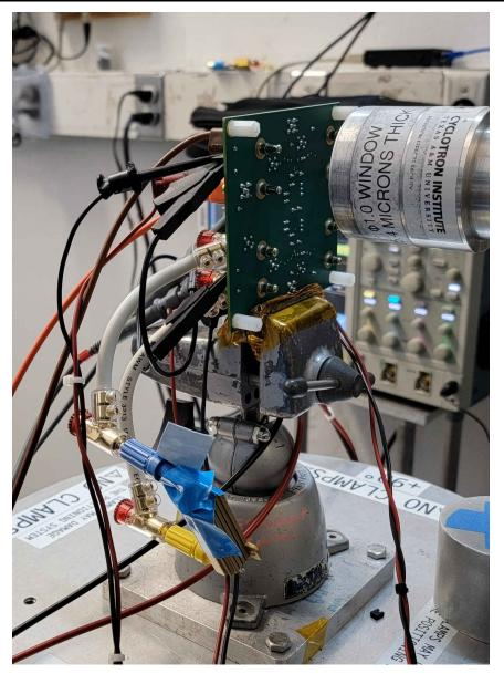
Figure 4-1. Photograph of the TPS7H2221-SEP Evaluation Board at the Texas A&M Cyclotron
