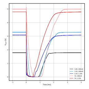
Figure 8-2. Typical VOUT<sub>SET</sub> at LET<sub>EFF</sub> = 42.7 MeV·cm<sup>2</sup>/mg
