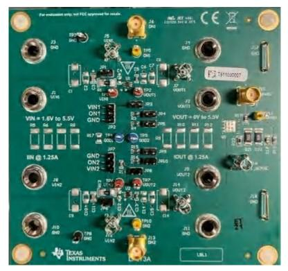
Figure 3-2. TPS7H2221-SEP Board Top View
