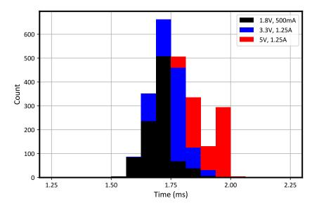
Figure 8-3. Histogram of the Transient Time for V<sub>OUT</sub> SETs at LET<sub>EFF</sub> = 46.8 MeV·cm<sup>2</sup>/mg
