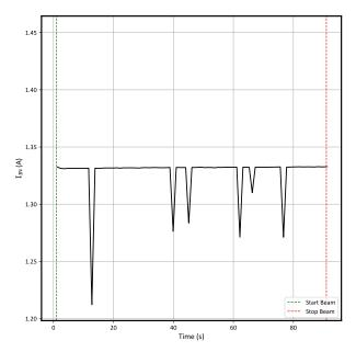
Figure 7-2. Current vs Time for Run # 4 (Enabled) for the TPS7H2221-SEP
