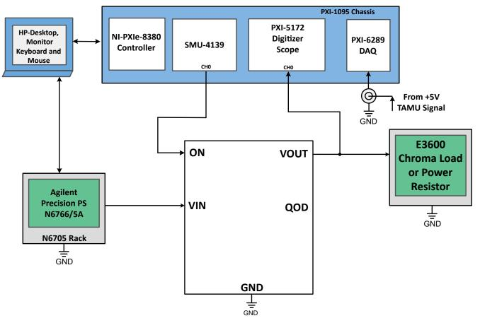
Figure 6-1. Block Diagram of SEE Test Setup With the TPS7H2221-SEP
