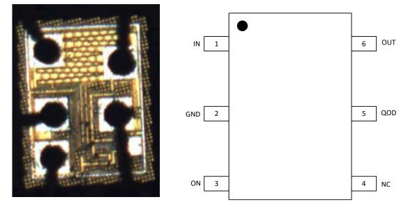
Note: Because the device is a flip chip, the package was delidded on the bottom to reveal the die face for all heavy-ion testing.
