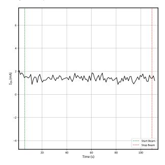
Figure 7-3. Current vs Time for Run # 5 (Disabled) for the TPS7H2221-SEP
