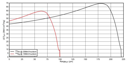
Figure 5-2. LET<sub>EFF</sub> vs Range for <sup>129</sup>Xe and <sup>109</sup>Ag at the Conditions Used for the SEE Test Campaign
