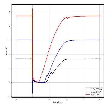
Figure 8-4. Typical VOUT<sub>SET</sub> at LET<sub>EFF</sub> = 46.8 MeV·cm<sup>2</sup>/mg
