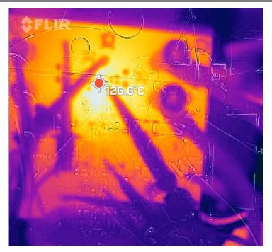
Figure 3-3. TPS7H2221-SEP Thermal Image for SEL
