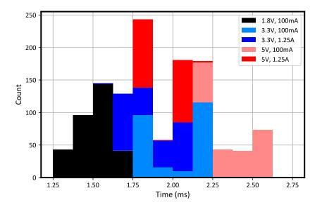
Figure 8-1. Histogram of the Transient Time for V<sub>OUT</sub> SETs at LET<sub>EFF</sub> = 42.7 MeV·cm<sup>2</sup>/mg
