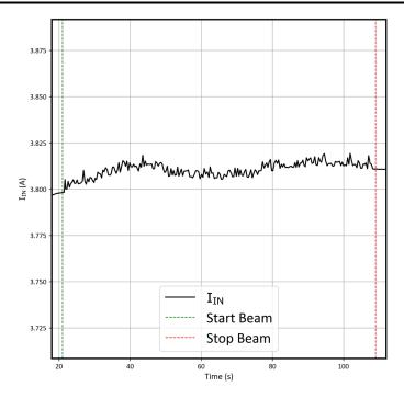
Figure 7-2. Current vs Time for Run # 6 (Enabled) for the TPS7H4003-SEP at T = 25°C
