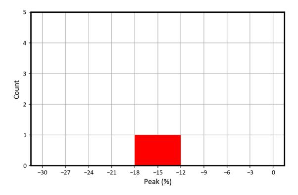
Figure 7-5. Histogram of the Normalized Amplitude for the Positive and Negative V<sub>OUT</sub> SETs on Run # 6
