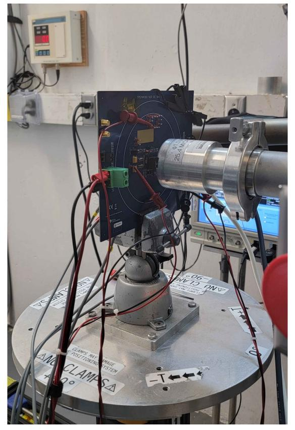
Figure 4-1. Photograph of the TPS7H4003-SEP Daughter Card Mounted in Front of the Heavy-Ion Beam Exit Port at the Texas A&M Cyclotron
