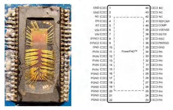
Figure 3-1. Photograph of Delidded TPS7H4003-SEP [Left] and Pinout Diagram [Right]
