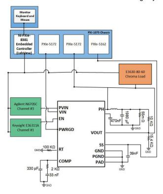
Figure 6-1. Block Diagram of SEE Test Setup With the TPS7H4003-SEP
