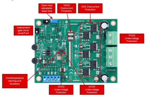
Figure 2-2. Protections Implemented on the DRV8329AEVM Applicable for Power Tools
