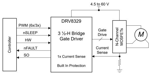
Figure 1-1. Simplified Schematic for DRV8329
