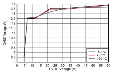
Figure 2-4. DRV8329 GVDD Voltage Over PVDD Voltage
